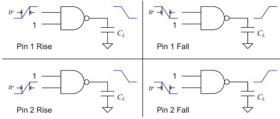
Fig. 2. Characterization of a NAND2 cell. The number of simulations required for characterization is identical to those of timing characterization.
