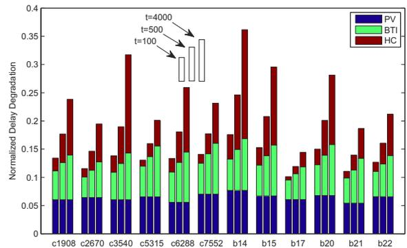
Fig. 9. Circuit degradation components from process variations (PV), BTI effects, and HC effects.
