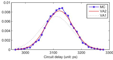
Fig. 7. The circuit delay PDF of benchmark b21 under variations.
