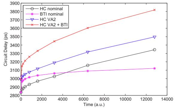
Fig. 8. Degradation vs. time of b21 for different degradation components.
