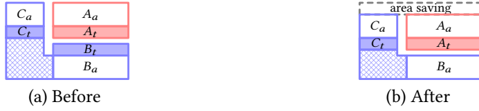
Fig. 12. Routes being preserved after removal of redundant tap vertices; Optimal well taps S = \{A_t, C_t\} .
