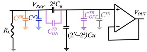
Fig. 2: Equivalent circuit of a charge-scaling DAC with the  $k^{\text{th}}$  bit set to 1 and all other bits set to 0.
