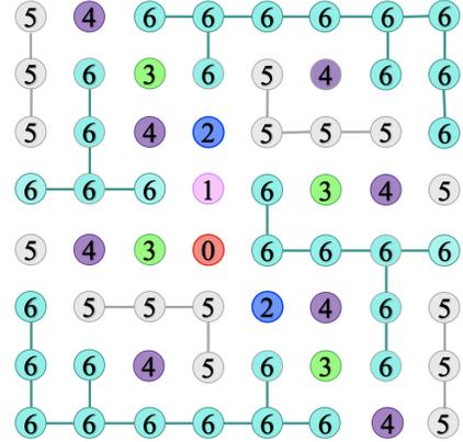
Fig. 7: Graph representation of connected capacitor groups.
