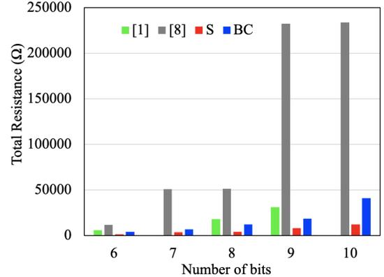
Fig. 13: Parasitic resistance for different bit DACs.
