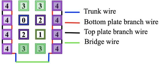
Fig. 8: Routing topology for  $C_4$ .
