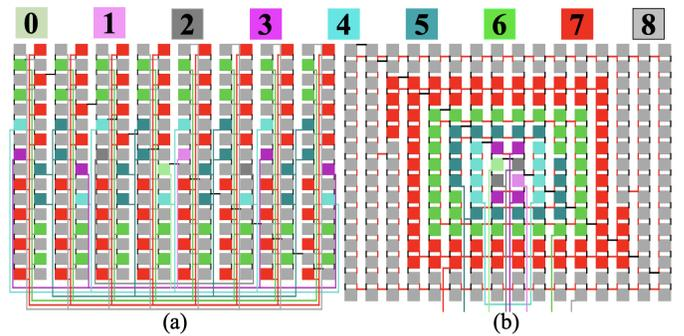
Fig. 14: CC layout in (a) [8] (b) spiral approach. High wirelength for [8] is inevitable: cells are spread for high dispersion.
