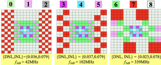
Fig. 12: 8-bit block chessboard layouts at various granularities.
