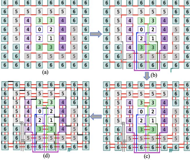
Fig. 9: Routing for a CC placement of a 6-bit DAC, (a) Connected capacitor groups formation [bottom-plate connections are shown in red], (b) Bottom plate routing, (c) Parallel wire routing, (d) Top-plate connections are shown in black.
