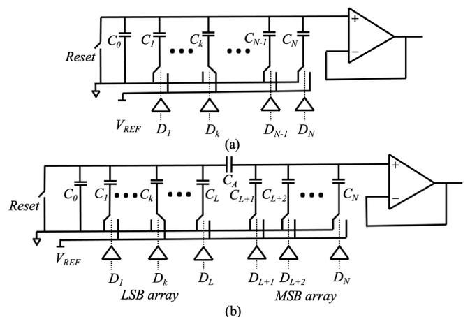
Fig. 1: Schematic circuit of a charge-scaling (a) binary, and (b) split DAC with the  $k^{\text{th}}$  bit set to 1 and all other bits set to 0.
