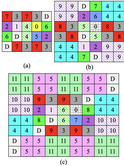
Fig. 11: Block chessboard placement for (a) 6-bit, (b) 8-bit, and (c) 10-bit split DAC.
