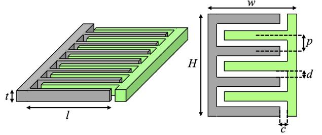
Fig. 5: Cross-section of a MOM capacitor in one metal layer.
