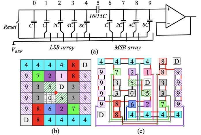
Fig. 10: CC placement and routing for a split DAC.
