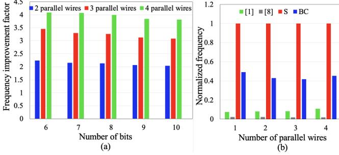
Fig. 15: 8-bit CC array with parallel wires: 3dB frequency improvements for (a) the spiral method. (b) all methods.
