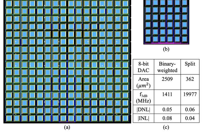
Fig. 16: CC layout of 8-bit (a) binary-weighted, and (b) split DAC, (c) comparison result table.
