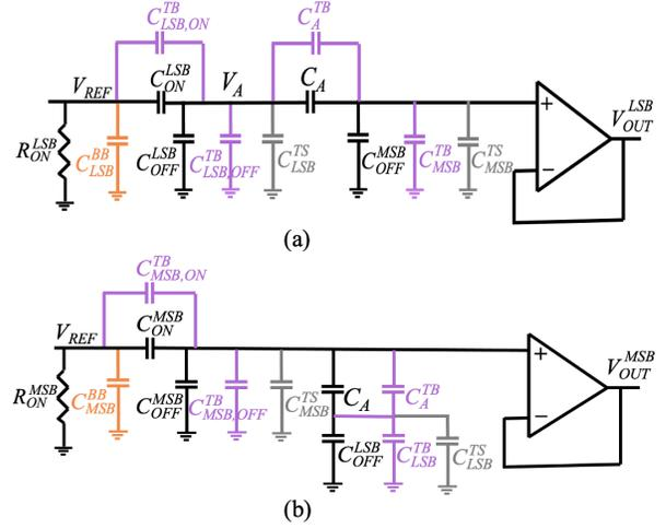
Fig. 3: Equivalent circuit of a split DAC with excitations applied to (a) the LSB array, and MSB excitations set to 0, (b) the MSB array, and the LSB excitations set to 0. The two cases are superposed to determine  $V_{OUT}^{LSB}$ .
