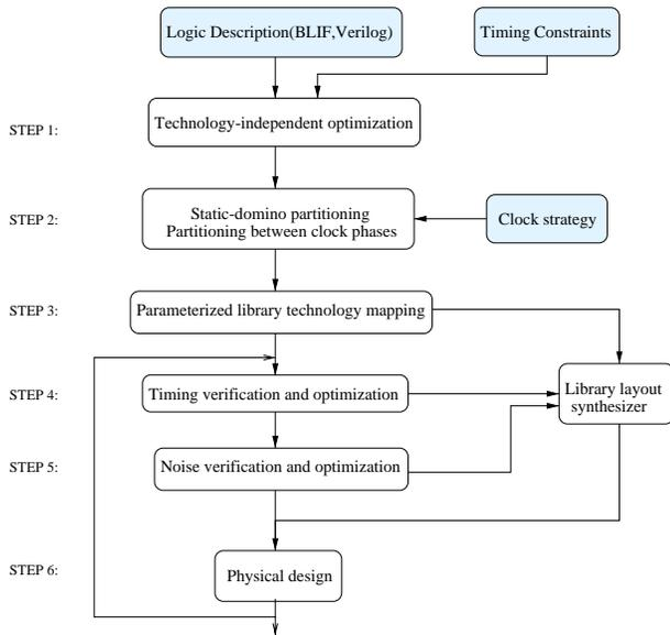
Fig. 2. Domino logic synthesis flow
