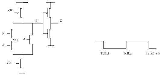
Fig. 1. A typical domino circuit
