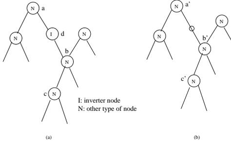
Fig. 5. Inverter elimination from the original network (a) in the twin network (b)
