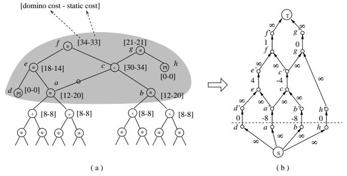
Fig. 8. Boolean network after mapping and candidate cut node decision
