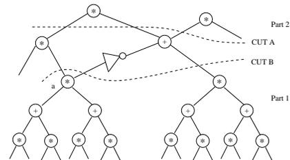
Fig. 4. An example for static-domino partitioning
