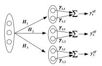
Fig. 1. Effective Channel for M = K = 3, N = 2 System
