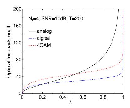
Fig. 5. Feedback length vs.  $\lambda$  for  $N_t=4$ ,  $\rho=10$  dB, T=200 symbols.
