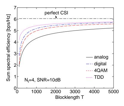
Fig. 3. Sum spectral efficiency vs. block length T.
