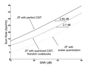
Fig. 2. Scalar quantization in MISO systems (M = 6, N = 1)
