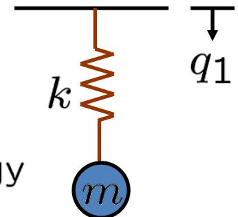
$$\frac{d}{dt} \left( \frac{\partial T}{\partial \dot{q}_1} \right) - \frac{\partial T}{\partial q_1} + \frac{\partial V}{\partial q_1} = F_1$$
