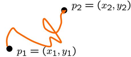
$$\begin{aligned} & (\frac{\partial}{\partial q_1} \hat{e}_1 + \frac{\partial}{\partial q_2} \hat{e}_2) \times (F_1 \hat{e}_1 + F_2 \hat{e}_2) \\ &= (\frac{\partial}{\partial x} \hat{i} + \frac{\partial}{\partial y} \hat{j}) \times (-kx\hat{i} + mg\hat{j}) \\ &= \left( \frac{\partial}{\partial x} (mg) - \frac{\partial}{\partial y} (kx) \right) \hat{k} = 0 \end{aligned}$$
