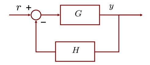
• If the O.L. T.F. G(s)H(s) has k poles in the RHP and  $n \geq m$  then, as  $\omega$  goes from  $-\infty$  to  $+\infty$ ,  $G(j\omega)H(j\omega)$  must encircle the -1 point k times in the CCW direction for stability Mathematically
