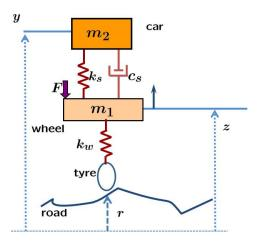
5. Consider the quarter car model shown, r, y and z denote the road height, car position and the wheel position respectively. F is a force acting on the wheel. Obtain a state space realization of the quarter car model with input being  $[r, F]^T$  and output being the car position y. Obtain the transfer functions from the input to the output.
