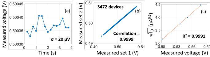
**Figure 2:** (a) Multiple measurements of the same device. (b) Repeatability test results. (c)  $\sqrt{I_D}$  vs.  $V_{GS}$ .
