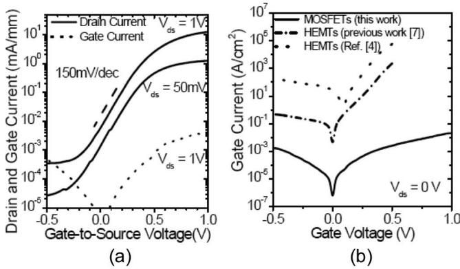
Fig. 2. Long buried-channel  $\text{In}_{0.70}\text{Ga}_{0.30}\text{As}/\text{In}_{0.52}\text{Al}_{0.48}\text{As}$  MOSFET with 10 nm MBE  $\text{HfO}_2$ ,  $L_g = 5 \mu\text{m}$ . (a) Subthreshold characteristics at  $V_{ds} = 50 \text{ mV}$  and 1 V, and gate leakage characteristics at  $V_{ds} = 1 \text{ V}$ . (b) Gate leakage characteristics at  $V_{ds} = 0 \text{ V}$ , with comparison to the previous HEMT devices [4], [7].
