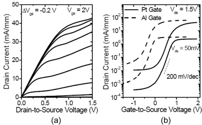
Fig. 4. (a) Output characteristics of a short-channel MOSFET with 7 nm ALD  $\text{Al}_2\text{O}_3$ ,  $L_g = 260$  nm, and a gate to source/drain contact distance of  $2.4 \mu\text{m}$ . (b) Subthreshold characteristics of an enhancement-mode and a depletion-mode short-channel MOSFET with  $L_g = 260$  nm and a gate to source/drain contact distance of  $2.4 \mu\text{m}$ .
