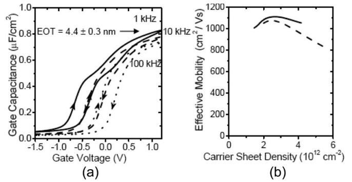
Fig. 3. (a) Gate capacitance versus voltage characteristics of a buried-channel MOSFET with 10 nm MBE  $\text{HfO}_2$  at frequencies of 1, 10, and 100 kHz. (b) Effective mobility versus carrier sheet density using 100 kHz  $C-V$  data, which were extracted for both (solid line) decreasing and (dashed line) increasing  $V_g$ .
