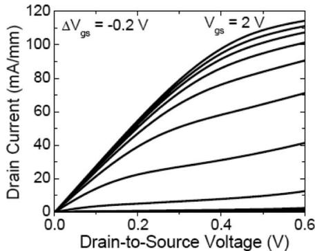
Fig. 5. Output characteristics of a short-channel MOSFET with 7 nm ALD  $\text{Al}_2\text{O}_3$ ,  $L_g = 260$  nm, and a gate to source/drain contact distance of  $0.4 \mu\text{m}$ .
