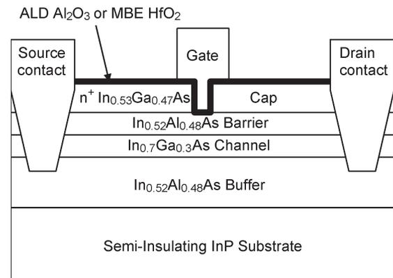
Fig. 1. Schematic cross-sectional diagram of an enhancement-mode In<sub>0.7</sub>Ga<sub>0.3</sub>As/In<sub>0.52</sub>Al<sub>0.48</sub>As MOSFET with 7-nm ALD Al<sub>2</sub>O<sub>3</sub> (short-channel device) or 10 nm MBE HfO<sub>2</sub> (long-channel device).
