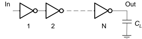
$$t_p = t_{p1} + t_{p2} + \dots + t_{pN}$$
