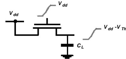
$$E_{0 \rightarrow 1} = C_L V_{DD} (V_{DD} - V_{Th})$$
