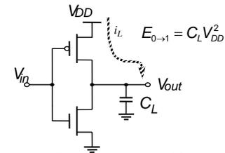
$$E_{0 \rightarrow 1} = \int_0^T P_{DD}(t) dt = V_{DD} \int_0^T i_{DD}(t) dt = V_{DD} \int_0^{V_{DD}} C_L dv_{out} = C_L V_{DD}^2$$
