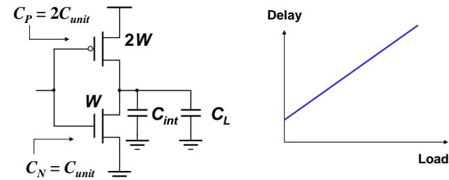
$$\begin{aligned} \text{Delay} &= kR_W(C_{int} + C_L) = kR_W C_{int} + kR_W C_L = kR_W C_{int} (1 + C_L / C_{int}) \\ &= \text{Delay (Intrinsic)} + \text{Delay (Load)} \end{aligned}$$
