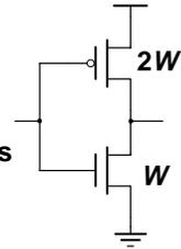
$$R_P = R_{unit} \left( \frac{W_P}{W_{unit}} \right)^{-1} \approx R_{unit} \left( \frac{W_N}{W_{unit}} \right)^{-1} = R_N = R_W$$
