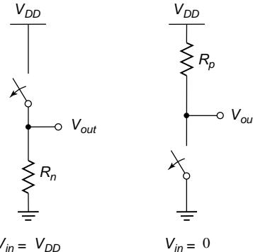
$$\begin{aligned}V_{OL} &= 0 \\V_{OH} &= V_{DD} \\V_M &= f(R_n, R_p)\end{aligned}$$
