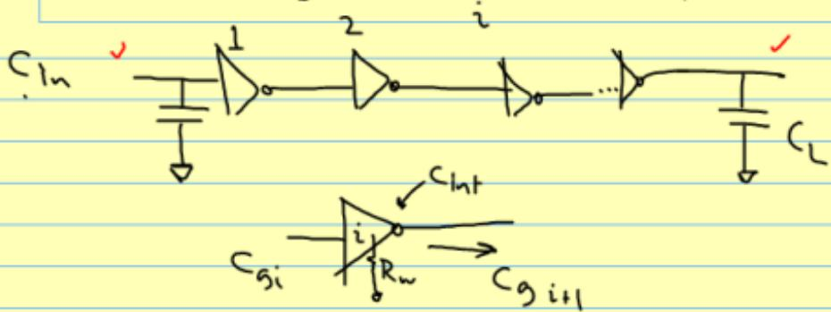
$$t_p = k R_w (C_{int} + C_{g,i+1}) = k R_w C_{int} \left(1 + \frac{C_{g,i+1}}{C_{int}}\right)$$
