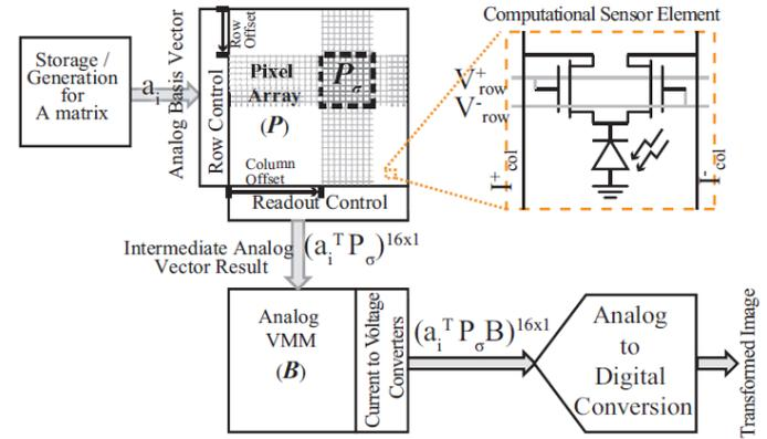
CMOS Separable Transform Image Sensor (Georgia Tech)
