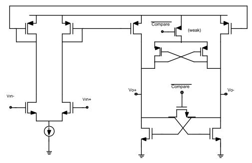
Comparator with pull-up scheme but no flashback compensaton
