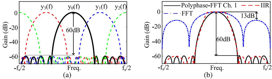
Fig. 12. (a) Frequency response of the P-FFT filter bank. (b) Comparison of frequency responses.
