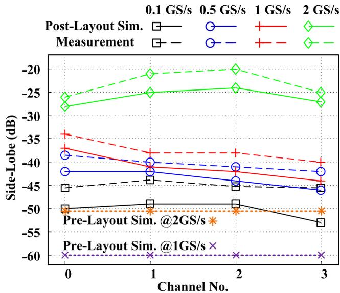
Fig. 22. Side-lobes per channel at different operating frequencies.
