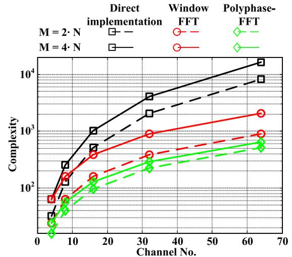
Fig. 11. Comparison of complexities for different structures.
