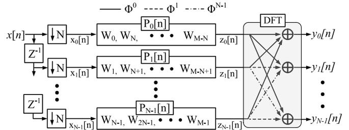
Fig. 8.  $N$ -channel P-FFT filter bank.
