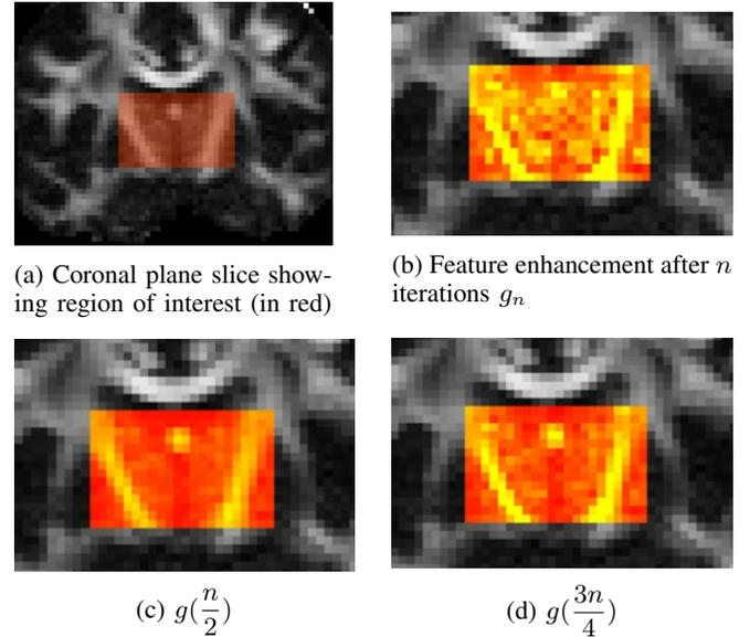
Fig. 4: Feature enhancement experiment (with backward Ricci flow) using MRI data. Number of iterations  $n = 40$ .
