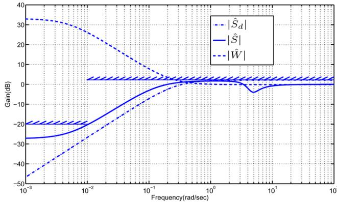
Fig. 3. Plots of  $|\hat{S}_d|$ ,  $|\hat{S}|$ ,  $|\hat{W}|$ , and the desired specification.
