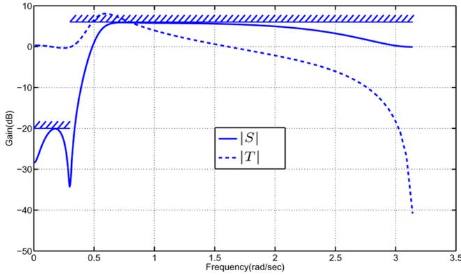
Fig. 2. Plots of  $|S|$ ,  $|T|$  and the desired specification.
