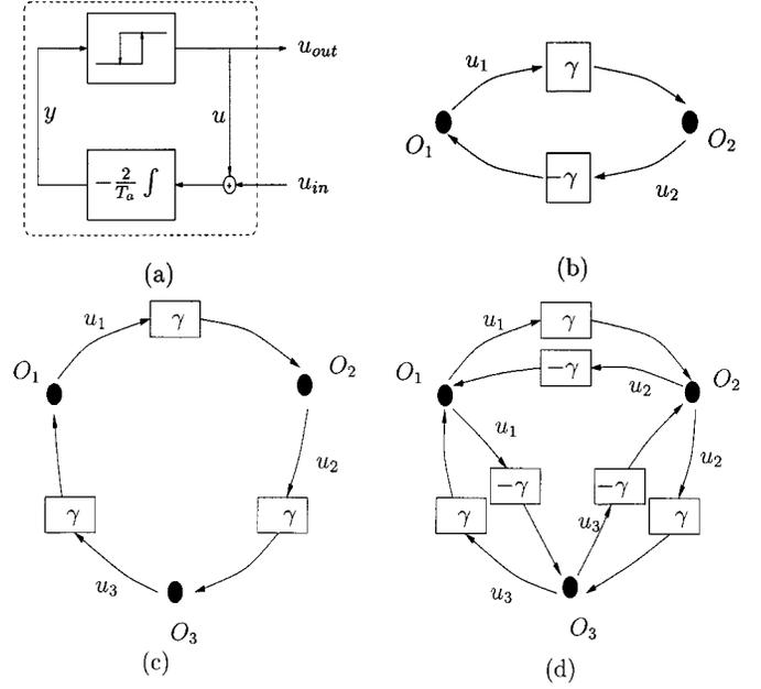
Fig. 11. Coupled relay oscillators. (a) single oscillator with input and output ports, (b) two member ring with gains  $\pm\gamma$ , (c) three member ring with one-way coupling, and (d) three member ring with two-way coupling.
