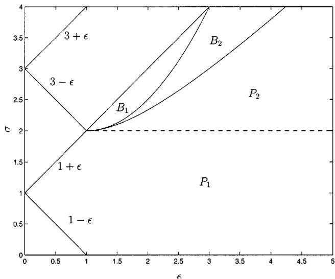
Fig. 10. Entrainment regions for the relay oscillator.
