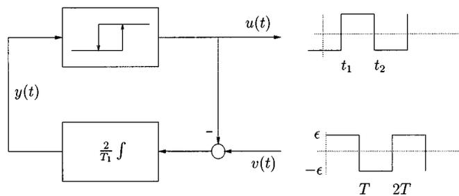
Fig. 9. Relay relaxation oscillator with a forcing input.
