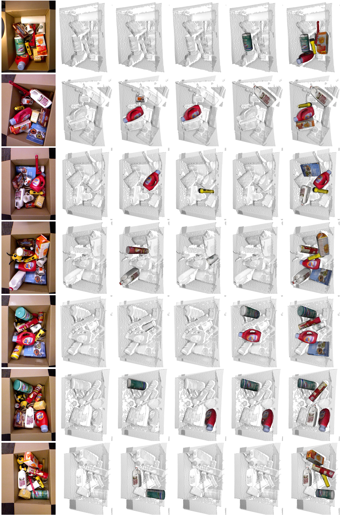
Figure 5.16. Selected pose estimation results of Hinterstoisser et al. (2012b) without the ICP (second row), Hinterstoisser et al. (2012b) with the ICP (third row), Papazov et al. (2012) (fourth row), Drost et al. (2010) (fifth row), and our approach (sixth row) in the real cluttered dataset. The first row shows the color image of the scanned RGB-D scenes. In these cluttered scenes, neither of approaches can recall more than half of the objects except our approach. Hinterstoisser et al. (2012b) without the ICP does not detect any objects, whereas it can recall one or two objects with the help of the ICP algorithm. Papazov et al. (2012) is also suffered from low recall in the cluttered scenes, and hence it detects at best one object per scene. Drost et al. (2010) works poorly because the low dimensional PPF feature does not give good matches between the model and the scene. Using the color information, CPPF is more discriminative so that pose results from the voting scheme are more likely to be the true positive poses.
