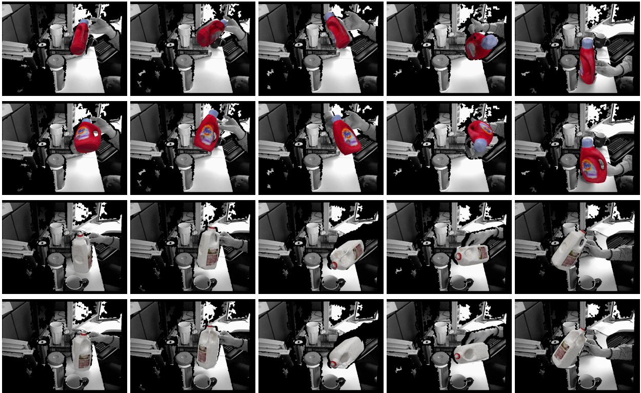
Figure 6.7. Tracking results on the “Tide” and “Milk” real sequences. For both sequences, the upper rows show the tracking results of our approach, while the lower rows present the results of the PCL tracking ( N = 1600 ). As the objects undergo significant variations in rotations, the PCL tracking suffered from false pose estimates. Thanks to multiple model renderings every time, our tracking reliably tracks the true poses of the objects. (Best viewed in color)
