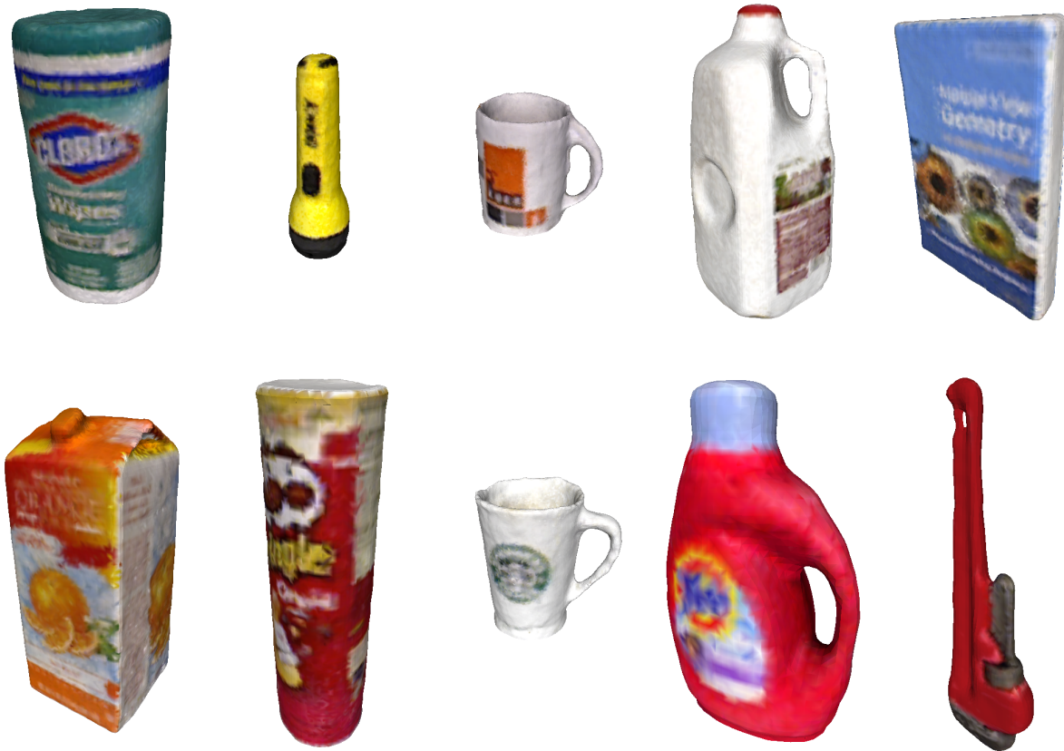
Figure 5.5. Polygonal mesh models of the test objects. Ten daily objects were chosen. Each object model is obtained by combining multiple views of object point clouds, followed by the Poisson reconstruction algorithm (Kazhdan et al. 2006). From left to right: Clorox, Flash, Kuka Mug, Milk, MVG Book, Orange Juice, Pringles, Starbucks Mug, Tide, and Wrench.
