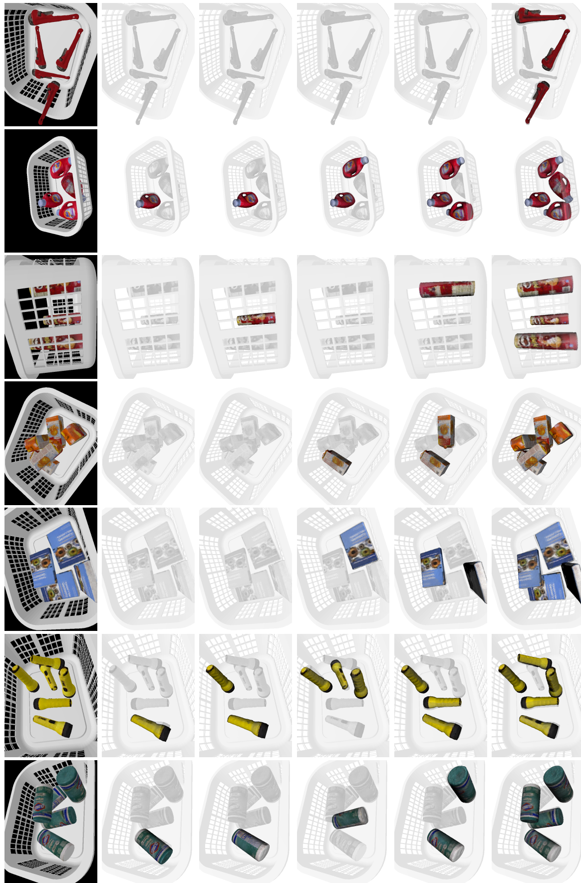
Figure 5.13. Selected pose estimation results of Hinterstoisser et al. (2012b) without the ICP (third row), Papazov et al. (2012) (fourth row), Drost et al. (2010) (fifth row), and our approach (sixth row) in the SOMI dataset. Our approach can handle the multiple instances scenario well, whereas Hinterstoisser et al. (2012b) and Papazov et al. (2012) fail to recognize multiple instances in most cases.
