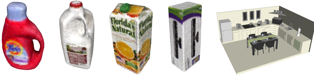
Figure 6.3. Mesh models for objects and kitchen. Object models were generated by fusing multiple RGB-D views, followed by running the Poisson reconstruction algorithm (Kazhdan et al. 2006). To generate a set of synthetic sequences, a kitchen model was downloaded from the Google 3D warehouse. From left to right, “Tide”, “Milk”, “Orange Juice”, “Kinect Box”, and “Kitchen”.
