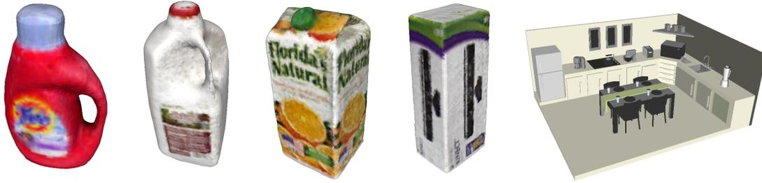
**Figure 6.3. Mesh models for objects and kitchen.** Object models were generated by fusing multiple RGB-D views, followed by running the Poisson reconstruction algorithm (Kazhdan et al. 2006). To generate a set of synthetic sequences, a kitchen model was download from the Google 3D warehouse. From left to right, “Tide”, “Milk”, “Orange Juice”, “Kinect Box”, and “Kitchen”.
