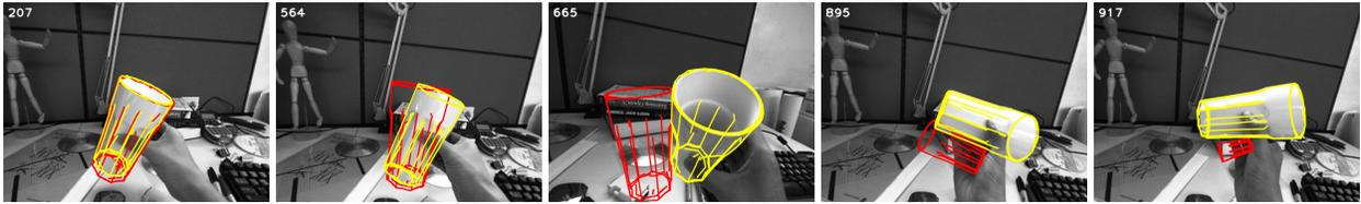
**Figure 4.2. Tracking results showing effectiveness of considering multiple hypotheses.** Results with 100 particles (yellow wireframe) and 1 particle (red wireframe) are shown in the sequence of the POKAL glass. Note that the yellow wireframe is well localized by calculating the mean of multiple hypotheses, while the red wireframe is drifted during entire tracking. The frame number is shown in the top left corner of each image.
