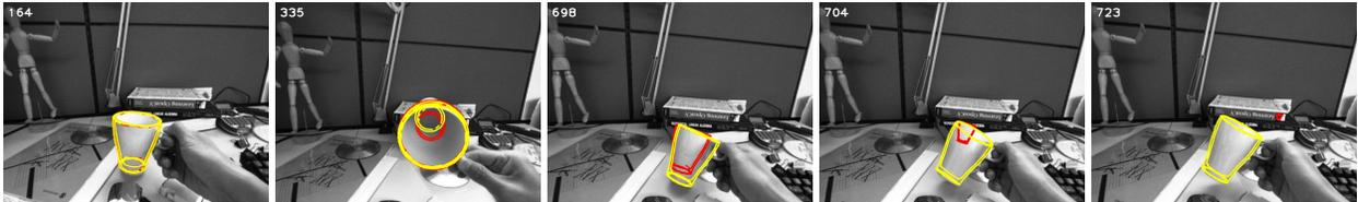
**Figure 4.3. Tracking results showing effectiveness of suppressing the rotating motion about the axis of symmetry.** Results with (yellow wireframe) and without (red wireframe) the suppression are shown in the sequence of the FARGRIK glass. Although they use the same number of particles and the parameters, the red wireframe starts to drift before the frame number 698 due to larger search space.
