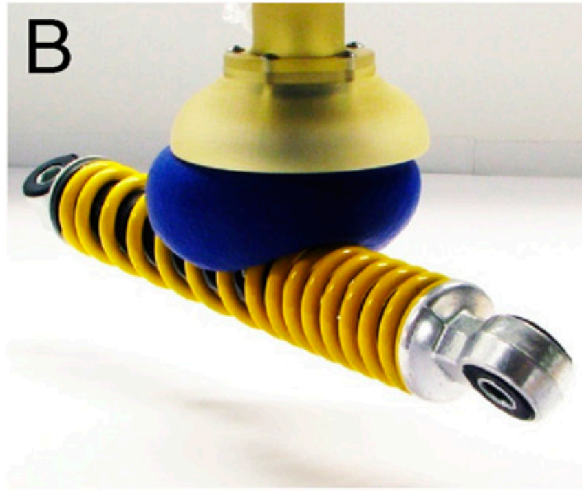
Jamming Gripper Brown et al., PNAS'10
