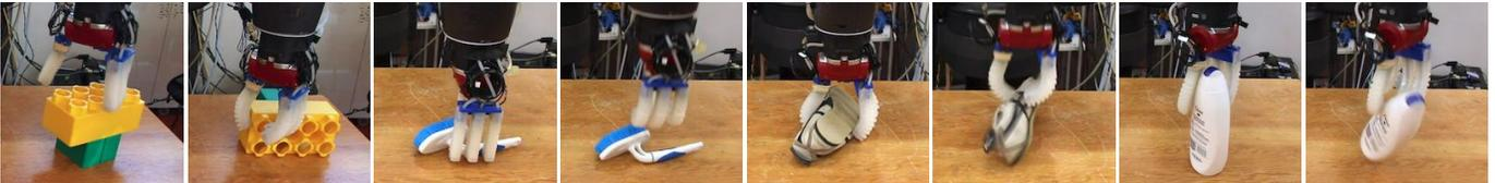
Fig. 10: **Unsuccessful grasps of the 3DCNN approach.** For each object, two images depict the pre-grasping and post-grasping situations. Although grasping directions and wrist orientations are right, final grasps are unsuccessful due to either the offsets in the gripper locations or challenging object poses.
