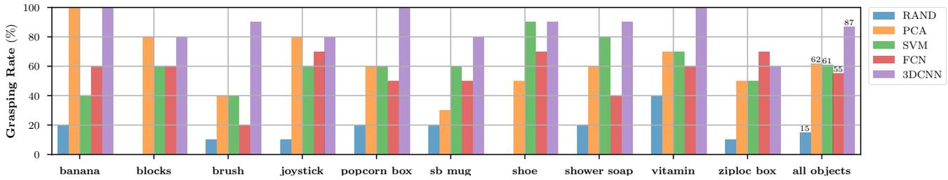
Fig. 7: **Grasping success rates on real robot.** The successful grasping rates of five approaches on the 10 test objects. The plot clearly shows the effectiveness of our approach, **3DCNN**, which achieves 87% of successful grasping for previously unseen objects.
