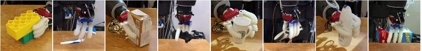
Fig. 8: **Successful grasps of the 3DCNN approach.** Our approach reliably grasps various objects even if these objects are unknown to the robot. The 3D CNN model generalizes for these previously unseen objects and enables our soft hands to approach to right directions and wrist orientations for grasping.
