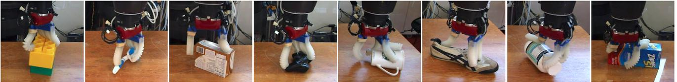
Fig. 9: **Unsuccessful grasps of the RAND approach.** Though our soft hands are compliant and adaptable to a certain degree of discrepancy, random trials often result in poor grasping as shown here. It clearly shows that an appropriate grasp pose is crucial even for these compliant soft hands.
