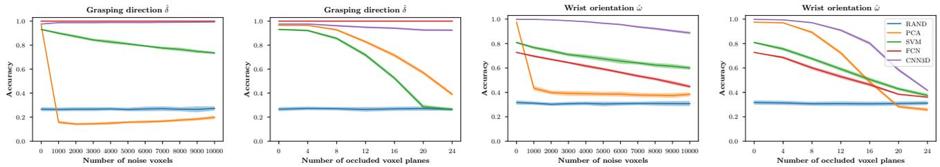
**Fig. 6: Prediction accuracy with respect to noise and occlusions.** The prediction accuracies of grasping direction  $\hat{\delta}$  and wrist orientation  $\hat{\omega}$  for five approaches are reported with different degree of noise and occlusions. We added artificial random noise voxels to the set of test voxel grids. We randomly removed some of consecutive voxel planes to mimic occlusions. The solid lines represent means and the shaded areas depict standard deviation.
