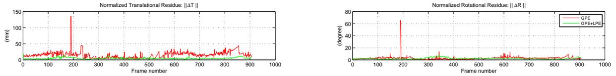
Fig. 9: Normalized residue plots of the book object in the general tracking test. The jitter and tracking failures result in a high residual.
