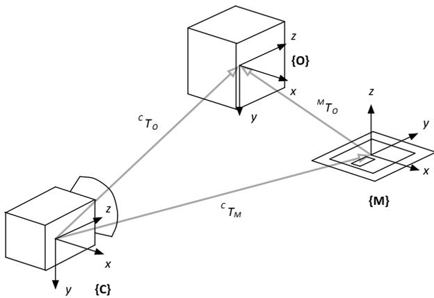
Fig. 10: Experimental setting and transformations between camera  $\{C\}$ , object  $\{O\}$  and marker  $\{M\}$  frames. We used AR markers to compute the ground truth pose.
