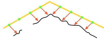
Fig. 7: Error calculation between projected model (yellow lines) and extracted edges (black tortuous lines) from the input image. Sample points (green points) are generated along the model per fixed distance, the error of each sampled point is calculated by the 1-D search along the direction orthogonal to the model edge.
