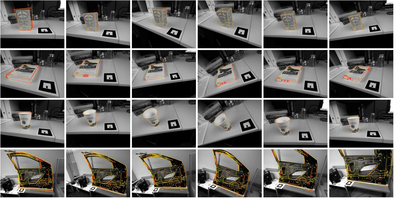
Fig. 6: Tracking results of the four targeted objects. From top to bottom, teabox, book, cup and car door. From left to right,  $t < 10$ ,  $t = 100$ ,  $t = 200$ ,  $t = 300$ ,  $t = 400$  and  $t = 500$  where  $t$  is the frame number. The very left images are results of the GPE.
