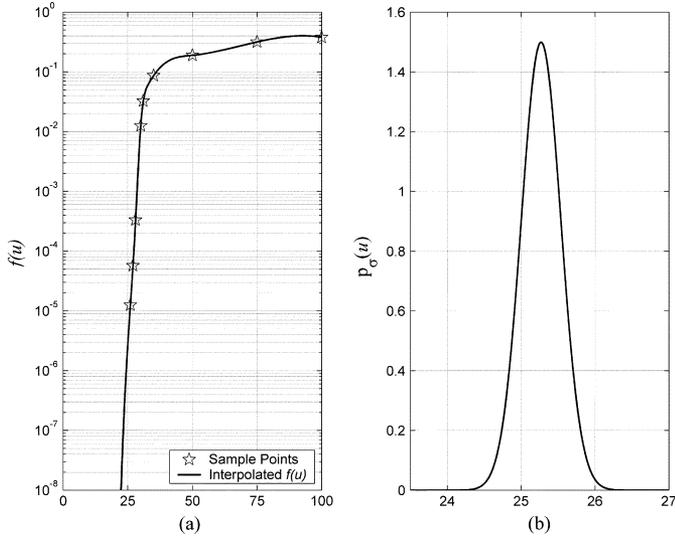
Fig. 2. Decomposition of the BER( $\sigma$ ) function into (a) cubic spline interpolation of the  $f(u)$  curve for the PR4 channel and (b) chi density function  $p_\sigma(u)$  for  $\sigma = 0.38$  (SNR = 9 dB) and  $n = 4509$ .
