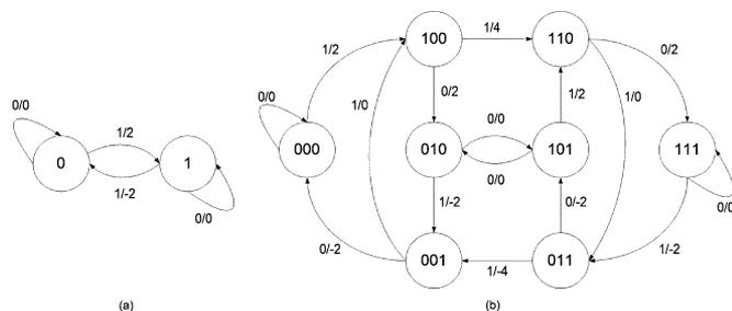
Fig. 5. State diagrams for (a) precoded PR4 channel and (b) precoded EPR4 channel.
