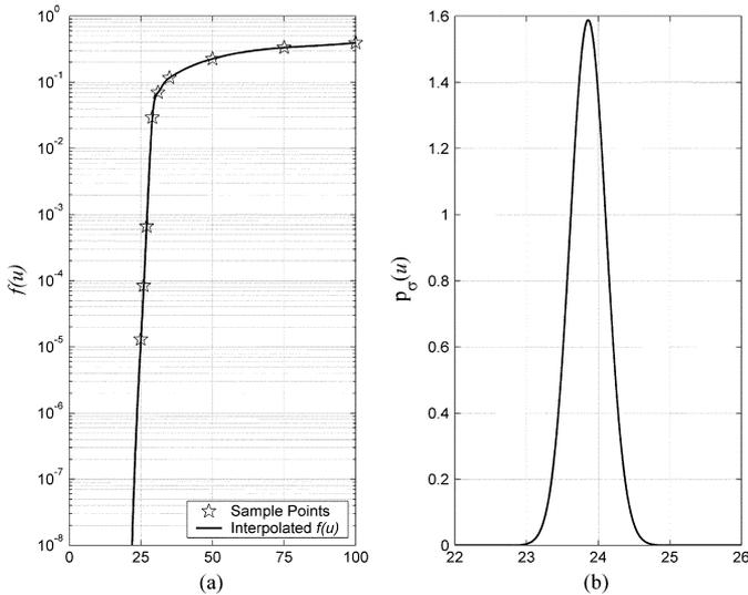
Fig. 3. Decomposition of the BER( $\sigma$ ) function into (a) cubic spline interpolation of the  $f(u)$  curve for the EPR4 channel and (b) chi density function  $p_\sigma(u)$  for  $\sigma = 0.35$  (SNR = 9.5 dB) and  $n = 4511$ .
