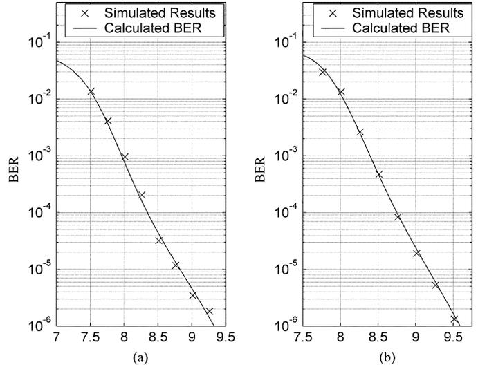
Fig. 4. Comparison of the simulated and calculated BER performance versus SNR for a rate 8/9 convolutional code after ten iterations on (a) PR4 channel and (b) EPR4 channel.
