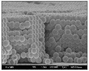
Tin oxide infiltrated spheres
