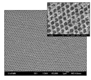
Inverse Opals composed of tinoxide nanoshells, 10-30 nm thick
