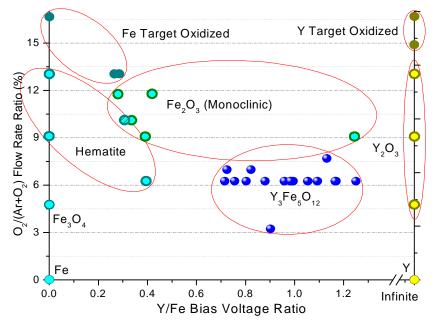
A wide processing window was identified for YIG grown on MgO with excellent optical quatilty.
