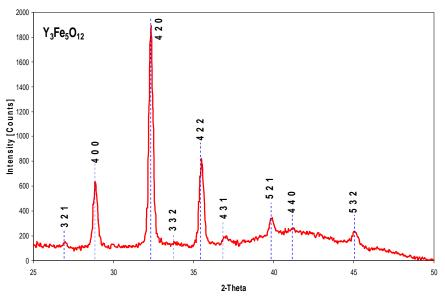
X-ray diffraction pattern of garnet film which was fabricated with multi-target RF sputter system.
