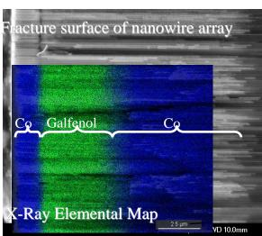
Electroplated thin films of Galfenol show grain morphology and composition using SEM and EDS, showing Fe<sub>81.2</sub>Ga<sub>18.8</sub>
