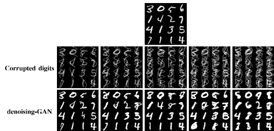
Fig. 2: The performance of trained generator for various level of corruption ( lc ) in denoising of unseen images. Top row: Ground truth digits. Middle row: corrupted digits with random sinusoidal, with a level of corruption from 1 to 5. Bottom row: the reconstructed digits.
