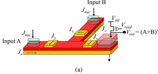
Fig. 4. (a) The design of a SkyLogic NOR2 gate.
