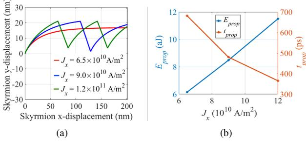
Fig. 6. (a) Skyrmion trajectory in the PMA-FM for various values of  $J_x$ . (b) Skyrmion propagation energy,  $E_{prop}$ , and propagation delay,  $t_{prop}$ , as a function of  $J_x$ . The material parameters used in this simulation are:  $M_{S,\text{PMA-FM}} = 1 \times 10^5$  A/m,  $K_{U,\text{PMA-FM}} = 8 \times 10^5$  J/m<sup>3</sup>, and  $\alpha = 0.25$ .
