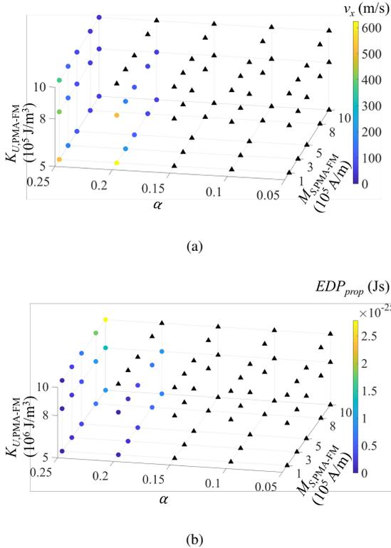
Fig. 7. For  $J_x = 9 \times 10^{10} \text{ A/m}^2$  and  $J_y = 5 \times 10^{11} \text{ A/m}^2$  (a) net velocity of the skyrmion,  $v_x$ , (b) energy-delay product during the propagation of the skyrmion,  $EDP_{prop}$ .
