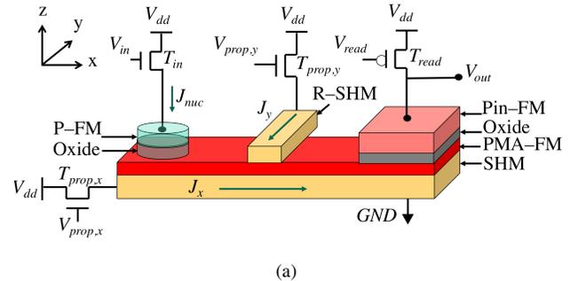
Fig. 1. (a) The structure of the SkyLogic device.
