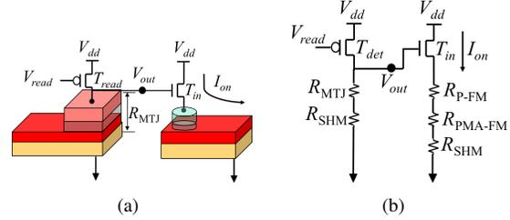
Fig. 5. (a) Two cascading SkyLogic devices (b) The equivalent circuit.
