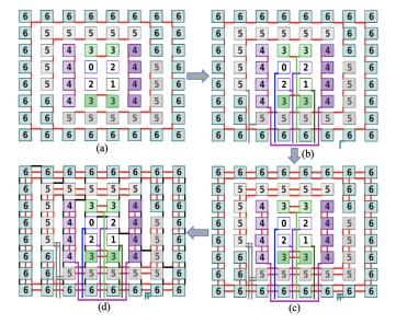
Fig. 9: Routing for a CC placement of a 6-bit DAC, (a) Connected capacitor groups formation [bottom-plate connections are shown in red], (b) Bottom plate routing, (c) Parallel wire routing, (d) Top-plate connections are shown in black.
