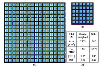
Fig. 16: CC layout of 8-bit (a) binary-weighted, and (b) split DAC, (c) comparison result table.
