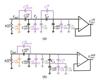
Fig. 3: Equivalent circuit of a split DAC with excitations applied to (a) the LSB array, and MSB excitations set to 0, (b) the MSB array, and the LSB excitations set to 0. The two cases are superposed to determine  $V_{OUT}^{LSB}$ .
