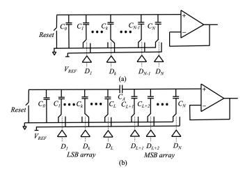
Fig. 1: Schematic circuit of a charge-scaling (a) binary, and (b) split DAC with the  $k^{\text{th}}$  bit set to 1 and all other bits set to 0.
