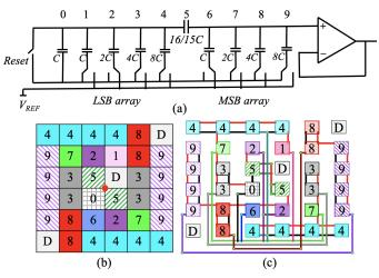
Fig. 10: CC placement and routing for a split DAC.
