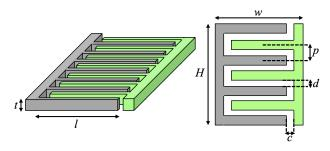
Fig. 5: Cross-section of a MOM capacitor in one metal layer.
