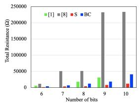
Fig. 13: Parasitic resistance for different bit DACs.
