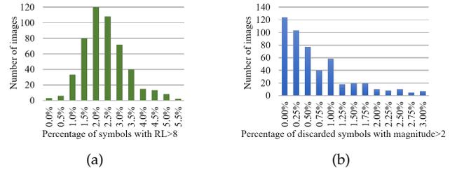
Fig. 6: The distribution of images based on the different percentage of symbols that cannot be covered by Class II representation for RL. (a) Discard the symbols with  $RL > 8$ . (b) The discarded symbols with the magnitude larger than 2.
