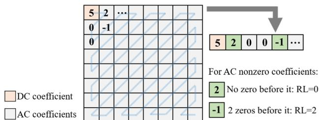
Fig. 2: The zigzag pattern that orders the DCT coefficients for storage.
