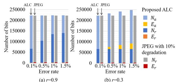
Fig. 21: Number of bits in reliable and approximate storage for the ALC scheme, as compared with VLC-encoded JPEG using reliable storage.
