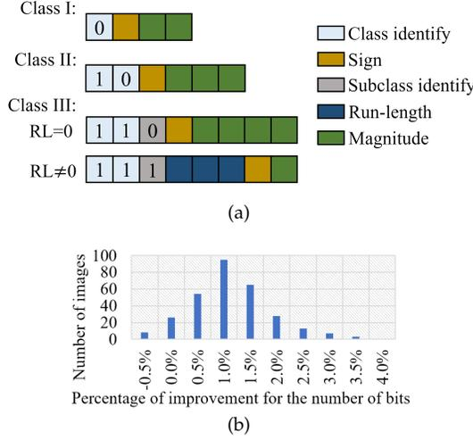
Fig. 14: (a) Bit assignment for three-class scheme (b) The distribution of images with different improvement in the total number of bits.
