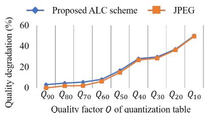
Fig. 20: Quality degradation for ALC scheme and JPEG with the same number of bits.
