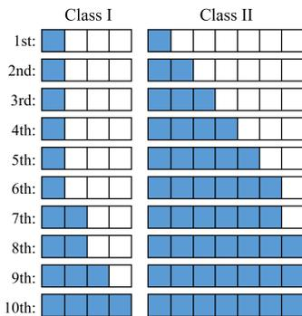
Fig. 12: The sequence of data partitioning patterns based on the importance order of bits in Class I and Class II, where the blue and white bits are stored in reliable and approximate storage, respectively.
