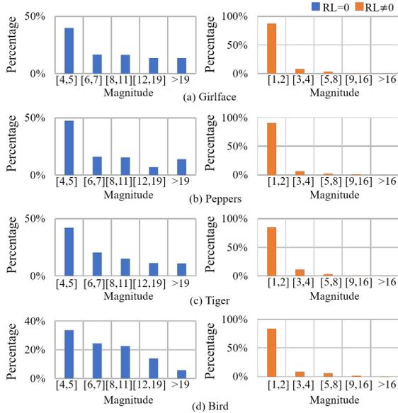
Fig. 5: A histogram of coefficient magnitudes for Class II symbols for a representative set of images, for  $RL = 0$  and  $RL \neq 0$ . The values in the x-axis for each class group several magnitude values when one more bit is added in the Class II magnitude field.
