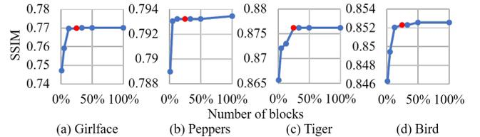
Fig. 10: The impact of using different number of blocks to decide the number of bits to be added to the first  $T$  AC codewords.
