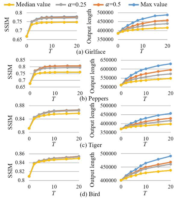
Fig. 9: The impact of using different methods to decide the number of bits to be added to the first  $T$  AC codewords.
