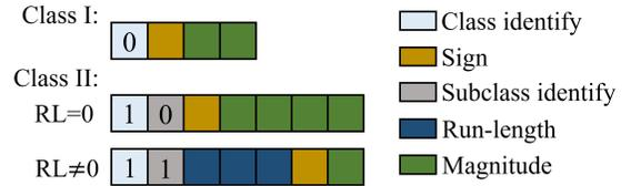
Fig. 4: Bit assignment for Class I and Class II symbols in the ALC scheme.
