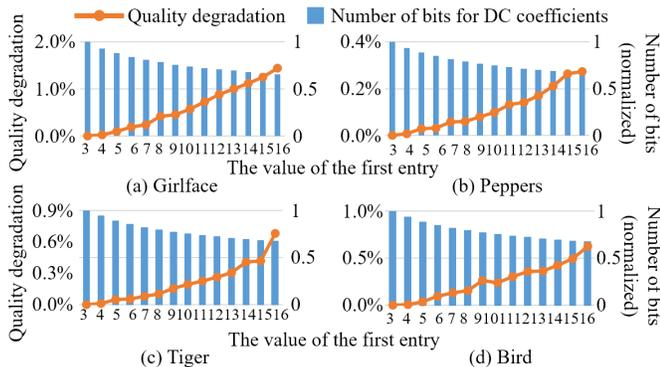
Fig. 24: Impact of the value of the first entry of the quantization matrix on the image quality and the number of bits for the DC coefficients.
