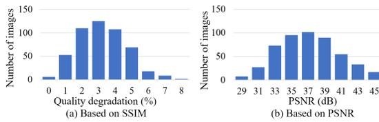
Fig. 17: The distributions of ALC inherent quality degradation based on SSIM and based on PSNR caused only by the approximate representation for 500 different images.
