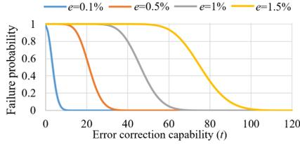
Fig. 16: Failure probability of error correction for different error rates,  $p$ , as a function of the error correction capability,  $t$ .
