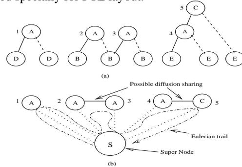
**Figure 11. Cluster formation: (a) A group of BDD nodes to be placed (b) The corresponding Eulerian graph**
