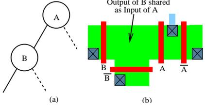
**Figure 5. An example of output diffusion-sharing: (a) A BDD (b) Its corresponding PTL implementation**
