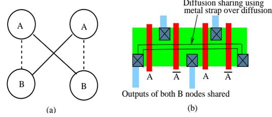
**Figure 6. A diffusion-sharing scheme for the case when two cofactors are shared: (a) A BDD (b) Its PTL implementation**
