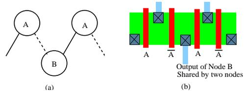
**Figure 4. An example of input diffusion-sharing: (a) A BDD (b) Its corresponding PTL implementation**
