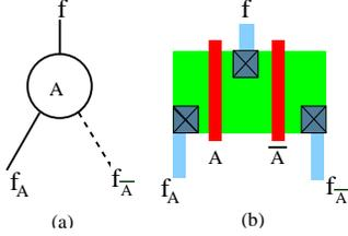
**Figure 1. Layout of a multiplexer: (a) A BDD node (b) Its corresponding layout**
