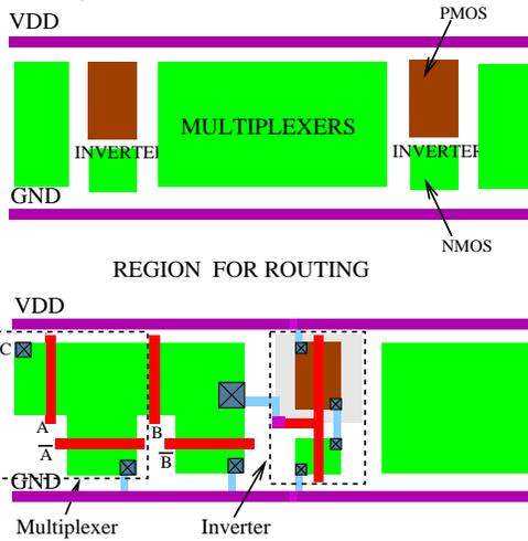
**Figure 2. A row-based layout scheme for PTL**
