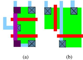
**Figure 3. Different multiplexers layout schemes: (a) with vertical transistors (b) with horizontal as well as vertical transistors**
