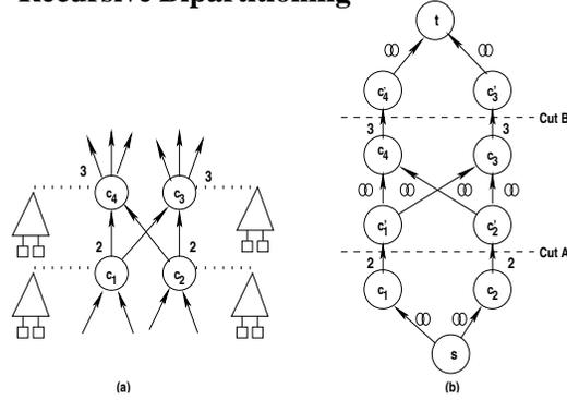
**Figure 9. Recursive bipartitioning: (a) A multi-level BDD network, (b) Its corresponding flow network**
