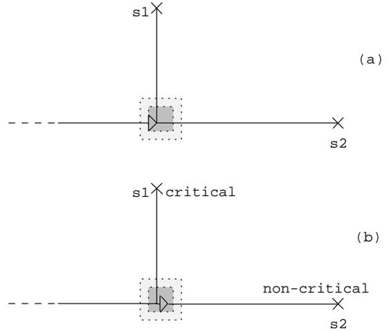
**Figure 5. Buffer insertion at an intersection of multiple paths according to the sink criticalities.**
