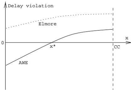
**Figure 4.** An example that Elmore delay and higher order AWE delay may result in different connection choice.
