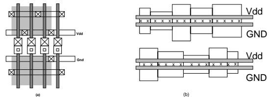
Figure 1: (a) A Flexible Macrocell (b) Macrocell Layout
