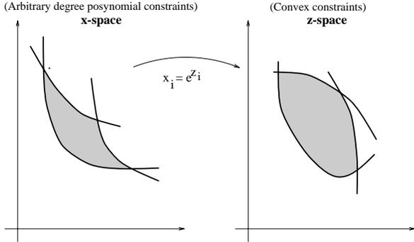
Figure 3: The transformation to convex programming.
