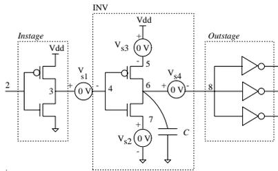
Figure 2: Calculating the power dissipation
