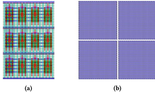
Figure 4: Parameterized primitive layouts for (a) a differential pair with transistors placed using common centroid, and (b) a  $2 \times 2$  MOM capacitor array.
