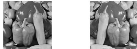
Fig. 9: The result of exact (left, PSNR=35.29) and approximate (right, PSNR=30.76) JPEG computations.
