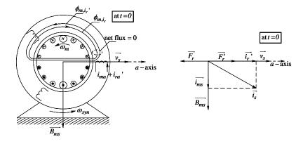
Neglecting the stator leakage impedance, at time t = 0, the stator-voltage space vector  $\vec{v}_s$  results in the magnetizing flux-density space vector  $\vec{B}_{ms}$ , by drawing magnetizing currents represented by the current space vector  $\vec{i}_{ms}$ . These magnetizing currents are animated by the equivalent winding in green. All these rotate at the synchronous speed  $\omega_{syn}$ .
