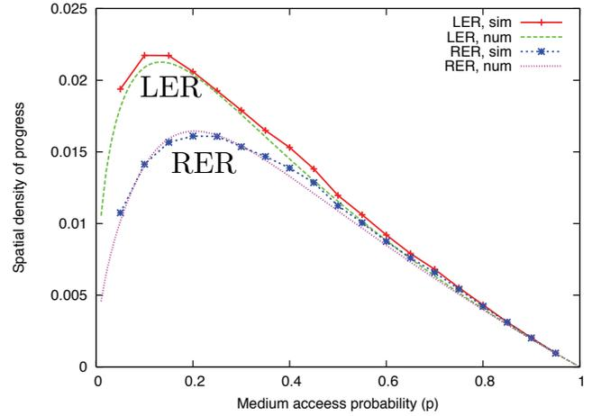
Fig. 2. Simulation and numerical results for spatial density of progress,  $h(\lambda, p)$ , for random edge routing (RER (12)) and longest edge routing (LER (16)), versus the medium access probability  $p$ . Optimal LER achieves 25% higher progress than optimal RER, with 33% fewer attempted transmissions.
