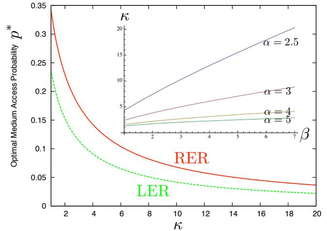
Fig. 4. Numerical results for the optimal medium access probability,  $p^*$ , for random edge routing (RER (13)) and longest edge routing (LER), versus  $\kappa$  (4). **Inset:**  $\kappa$  versus the SINR requirement  $\beta$  for pathloss exponents  $\alpha = \{2.5, 3, 4, 5\}$ .
