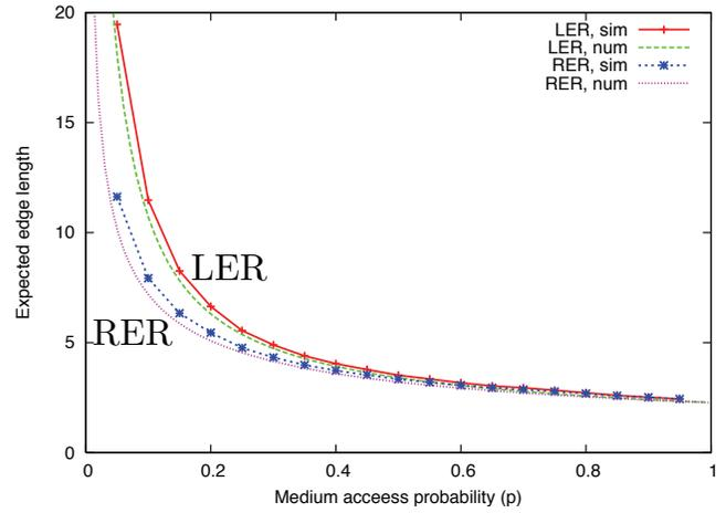
Fig. 3. Simulation and numerical results for expected edge length,  $\mathbb{E}[L], \mathbb{E}[L^{\max}]$ , for random edge routing (RER (11)) and longest edge routing (LER (15)), versus the medium access probability  $p$ . The numerical edge lengths are unbounded as  $p \rightarrow 0$  on account of the no noise assumption.
