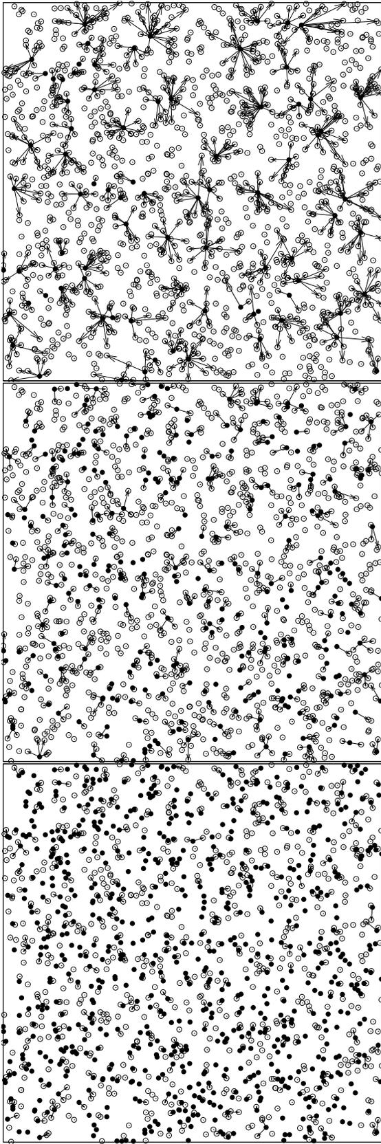
Fig. 1. A realization of the spatial Aloha graph for  $p = 0.05$  (top),  $p = 0.20$  (middle), and  $p = 0.50$  (bottom). Transmitters are denoted by  $\bullet$ , receivers by  $\circ$ , and an edge indicates an SINR above  $\beta = 1$ . The square arena has a side length of  $200\sqrt{2}$  meters and there are approximately 1600 nodes. The pathloss exponent is  $\alpha = 3$  and the noise power is  $\eta = 10^{-6}$ . Zooming in on the bottom plot reveals many very short edges.
