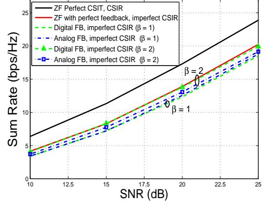
Fig. 1. Quantized vs. Analog Feedback with Imperfect CSIR.
