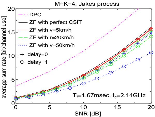
Fig. 3. Rates with feedback delay and Jakes' correlation.
