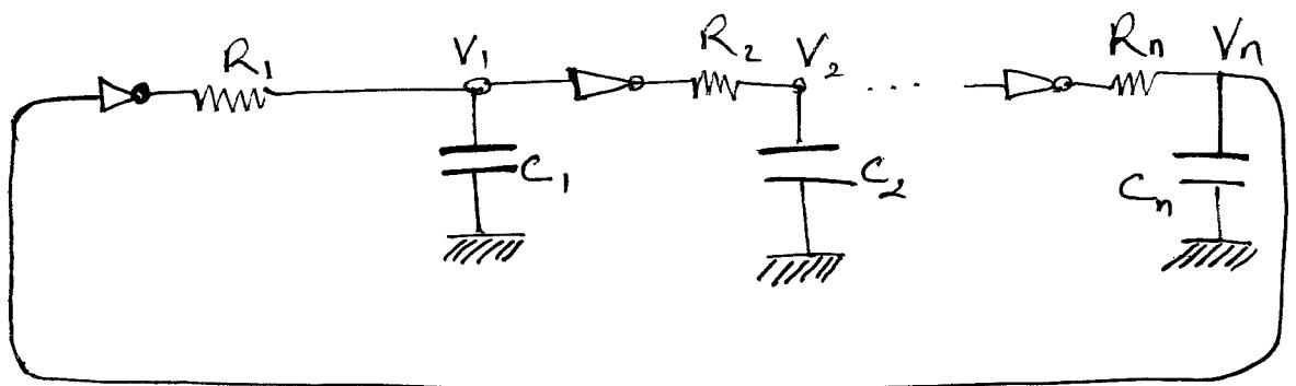
$$\left. \begin{array}{l} R_1 C_1 \dot{V}_1 = -V_1 - h_n(V_n) \\ R_2 C_2 \dot{V}_2 = -V_2 - h_1(V_1) \\ \vdots \\ R_n C_n \dot{V}_n = -V_n - h_{n-1}(V_{n-1}) \end{array} \right\} \text{nonlinearities}$$
