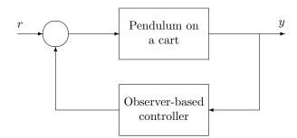
Note: you can use the MATLAB command feedback to solve this problem. Since this command assumes negative feedback (and here the negative sign is already included in the controller), you will need to multiply the system in the feedback loop with -1 when using this command. If you are unsure how this command works type help feedback, and check it first on a simple example for which you can easily determine the answer by hands.
