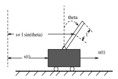
Figure 1: Inverted pendulum on a cart.
