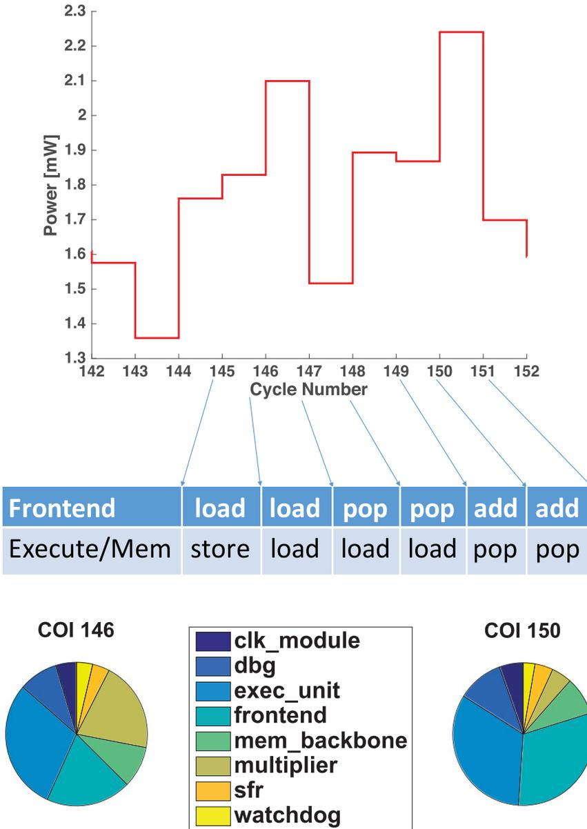
Fig. 17. A snapshot of instantaneous power profiles for *mult* at two different COIs where peaks occur. Our technique analyzes the instructions in the pipeline (top) to find each COI’s culprit instructions that cause the peak power in each pipeline stage along with the per-module peak power breakdown (bottom) to identify which instructions in which microarchitectural modules are responsible for a peak.
