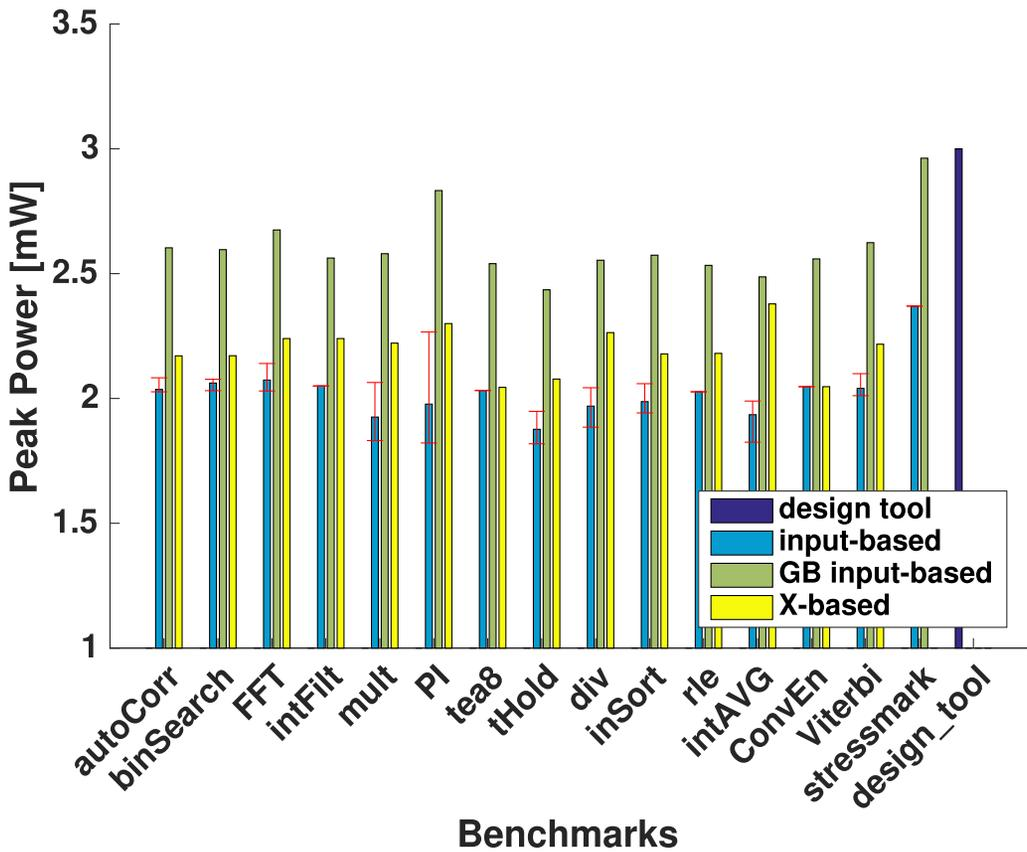
Fig. 19. Our X-based technique for determining peak power requirements provides the most accurate (least conservative) guaranteed bound on peak power.
