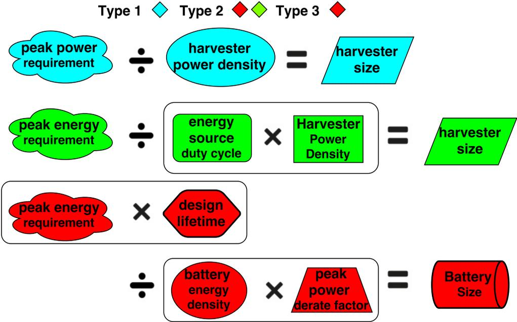
Fig. 3. Harvester and battery size calculations for Types 1, 2, and 3 ULP systems depend on peak power and energy requirements.
