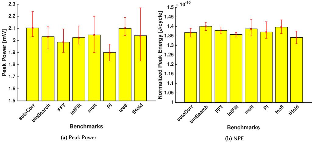
Fig. 7. The peak power and normalized peak energy (normalized to an application’s runtime in cycles) of a ULP processor are different for different applications and different inputs. The bars represent average across all inputs; error bars show the range of input-induced peak and average power variations. Measured variation between multiple runs of the same application and same input is less than 2%.
