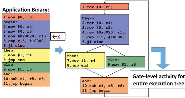
Fig. 10. Symbolic input-independent gate activity analysis involves using unknown logic values for application inputs to characterize application-induced processor behavior for all possible executions of an application.
