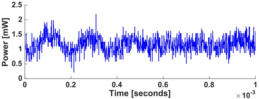
Fig. 8. Measured instantaneous power of MSP430F1610 for the *mult* benchmark is significantly lower, on average, than both the rated and observed peak power for the application.
