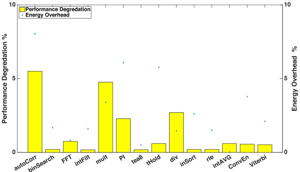
Fig. 24. Performance degradation and energy overhead introduced by peak power optimizations is small (average: 1%).
