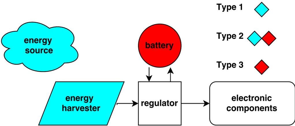
Fig. 1. ULP systems are commonly powered by energy harvesting, battery, or a combination of the two, in which harvesters are used to charge the battery.
