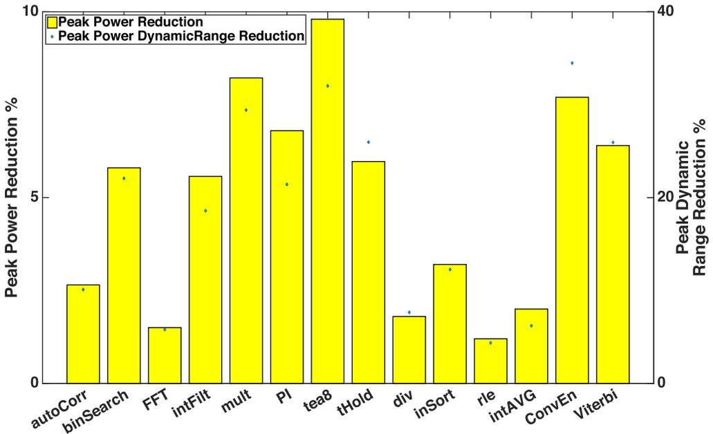
Fig. 22. Peak power reduction (left axis) and peak power dynamic range reduction (right axis) achieved by optimizations. These reductions are enabled by our analysis tool and provide further reduction in energy harvester size.
