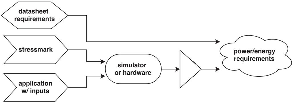
Fig. 4. The conventional methodology for sizing energy harvesting and storage components involves determining peak power and energy requirements for a processor and selecting components that will provide enough power and energy to satisfy the requirements over the lifetime of the system.
