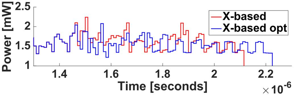
Fig. 23. A snapshot of instantaneous power profiles for mult before and after optimization.
