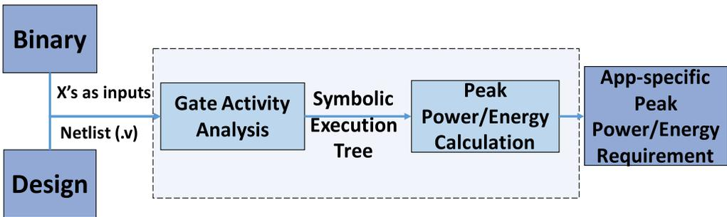
Fig. 9. Our technique performs input-independent activity analysis that enables determination of accurate peak power and energy requirements for a ULP processor.
