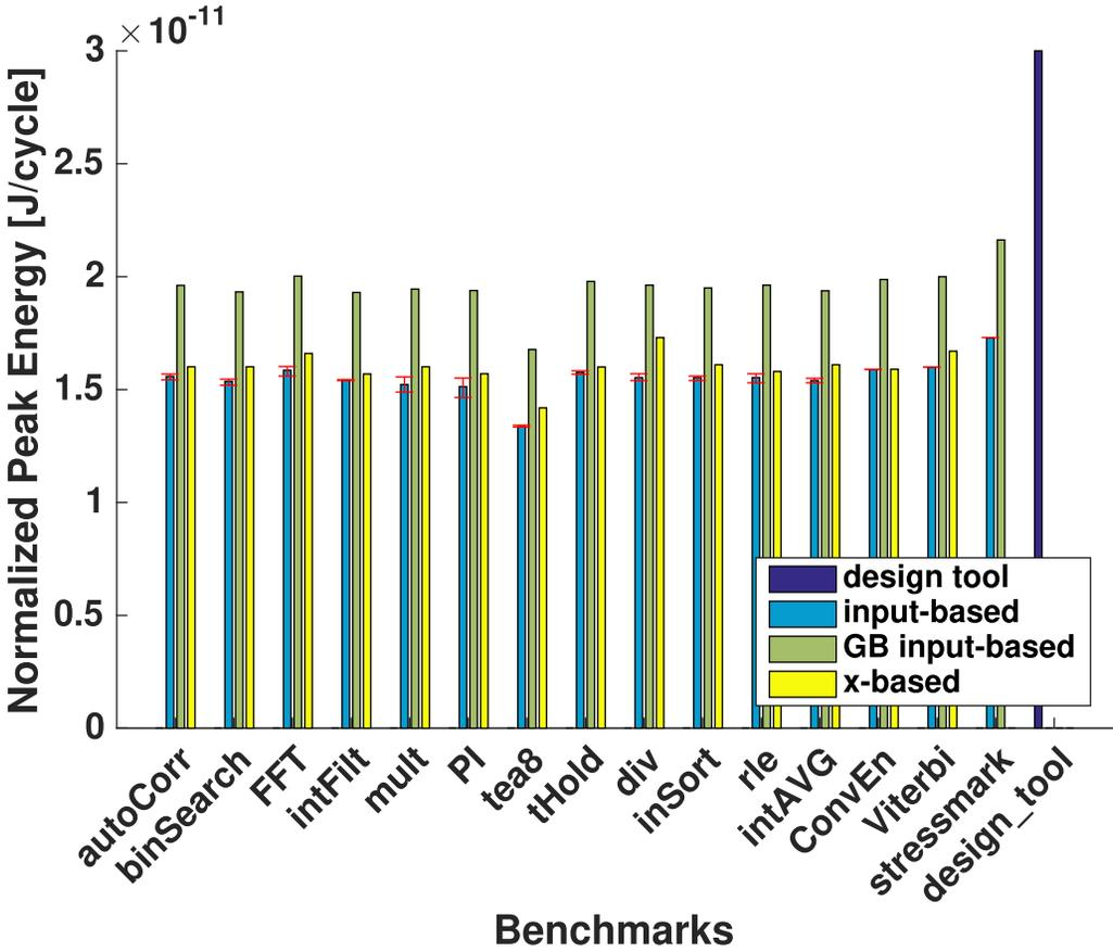
Fig. 20. Our X-based technique for determining peak energy requirement (normalized to application runtime in cycles, i.e., the peak average power) is more accurate than existing conventional techniques.
