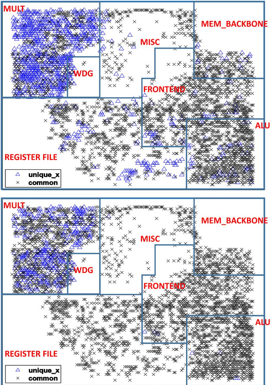
Fig. 15. Toggled gates for *mult* with low-activity inputs (top) and high-activity inputs (bottom) compared against potentially toggled gates identified by X-based analysis. X-based simulation marks all gates that can potentially toggle for an application for all possible inputs. This set of gates ( $\text{unique\_x} \cup \text{common}$ ) is a superset of the gates that toggle during an input-based application execution (common).
