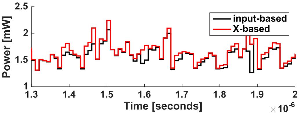
Fig. 16. The X-based peak power trace generated by our technique for an application provides an upper bound on all possible input-based power traces for the application (result shown for *mult*).
