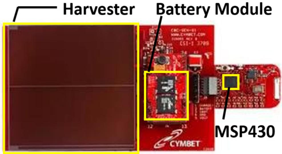
Fig. 2. In most ULP systems, like this wireless sensor node, the size of the battery and/or energy harvester dominates the total system size.
