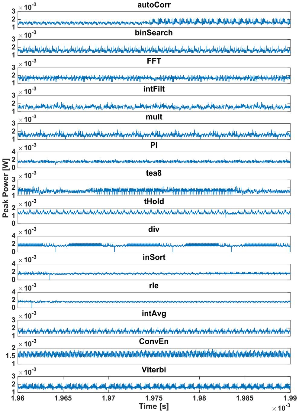
Fig. 14. The per-cycle peak power varies significantly over the course of an application, showing that the worst-case average power can be significantly lower than peak power. Therefore, the peak energy can be significantly lower than the product of peak power and application runtime would suggest.
