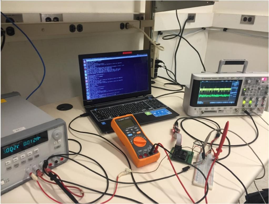
Fig. 6. The test setup used to measure peak and average power on a ULP processor (MSP430).
