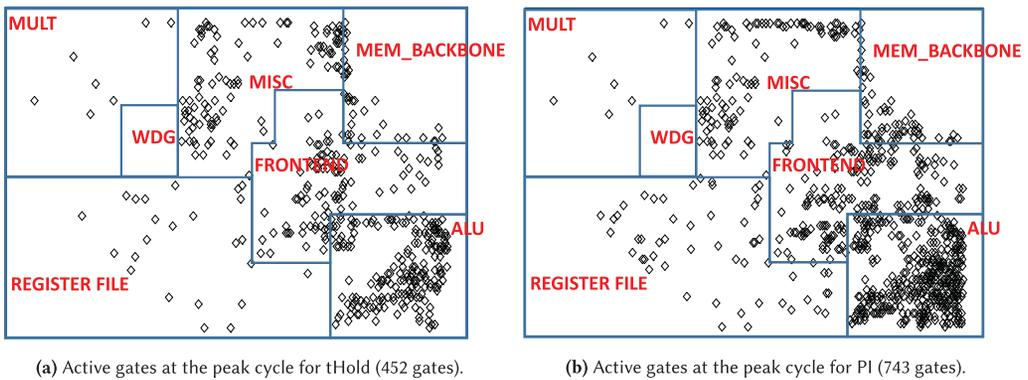
Fig. 5. Different applications can have different activity profiles, resulting in peak power and energy requirements that are application specific.
