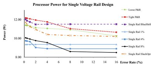
Fig. 9. This figure demonstrates the power benefit of a processor that is designed to allow errors in the arithmetic units over a processor that is designed for correctness. All modules in the processor operate at the same voltage. Razor is used to correct errors in non-arithmetic units.
