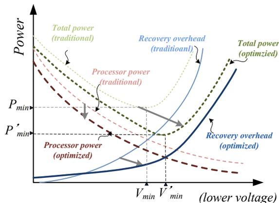
Fig. 1. Design for a target error rate ensures that the target error rate is exceeded at a substantially lower voltage of an already lower power processor, significantly reducing the power consumption at the target error rate, lowering recovery overhead for hardware-based error tolerance and decreasing degradation in output quality for software-based error tolerance.
