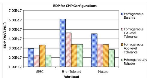
Fig. 10. The heterogeneously reliable CMP is able to adapt to the needs of the applications to provide power efficiency for a diverse set of applications.
