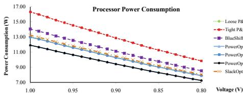
Fig. 6. The power of a processor design at a given voltage shows the relative ordering of designs in terms of power overhead.
