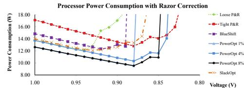
Fig. 7. The benefit of designing a processor to produce errors then correcting them with an error tolerance mechanism over designing for correctness and then relaxing the correctness guarantee can be significant. Results are shown for processors with Razor.
