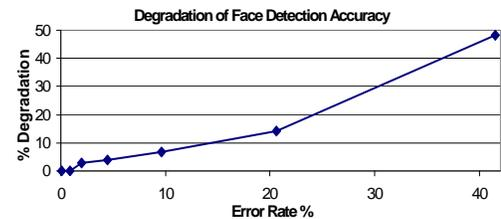
Fig. 8. The figure above shows how the detection accuracy for the face detection application degrades as the error rate of the processor is increased. Even at some non-zero error rates, maximum output quality can be achieved.
