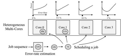
Fig. 3. The heterogeneously reliable CMP matches each application to the core that has minimum power for the application’s reliability requirement.
