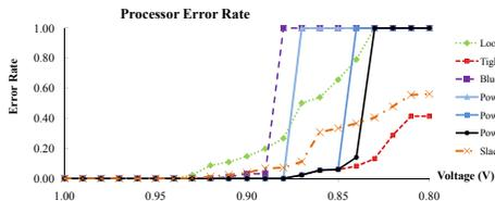
Fig. 5. The voltage at which a design reaches its target error rate determines how much power can be reduced through voltage scaling.
