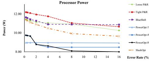
Fig. 4. Processors optimized for different error rate targets consume the least power out of all alternative designs, especially around the error rate target for which they were optimized.
