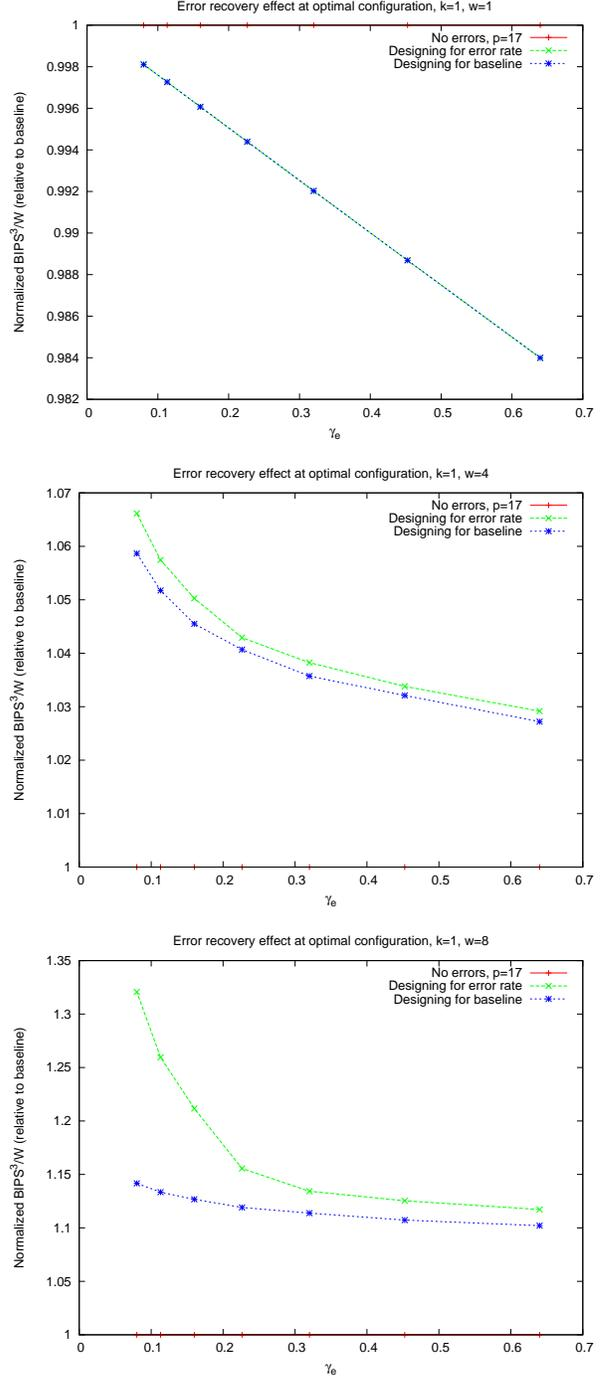
Fig. 5. The benefit of re-optimizing an architecture depends strongly on the error rate vs voltage relationship. Architectures consisting of circuits seeing fewer errors at a particular voltage (bottommost figure) will see the most benefits from re-optimization.
