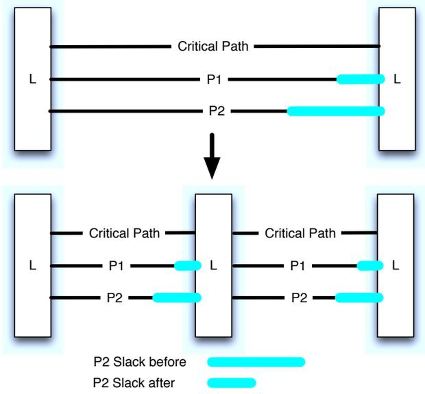
Fig. 1. The effect of pipelining on the slack of a design (the highlighted portion denotes the path slack). When a logic stage is pipelined, the absolute length of the timing paths, and therefore the amount of slack per stage, is reduced. This causes more errors for a given absolute reduction in voltage.
