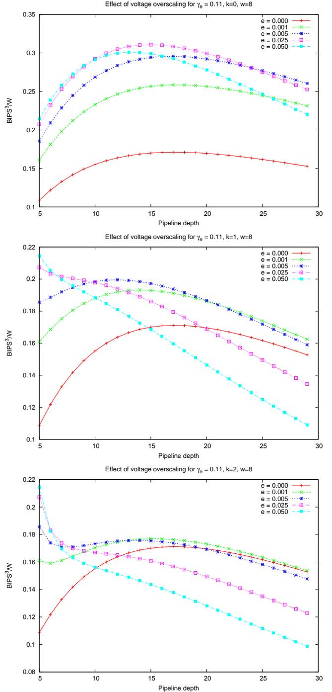
Fig. 3. Error resilient designs see greater benefits from shorter pipelines as the available path slack decreases faster due to pipelining. From top to bottom,  $k=0,1,2$
