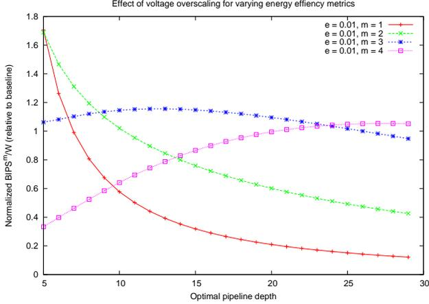
Fig. 4. Benefits of error resiliency improve for energy efficiency metrics dominated by power. The figure shows the benefit of error resiliency for  $m=1,2,3,4$  ( $BIPS^m/W$ ).
