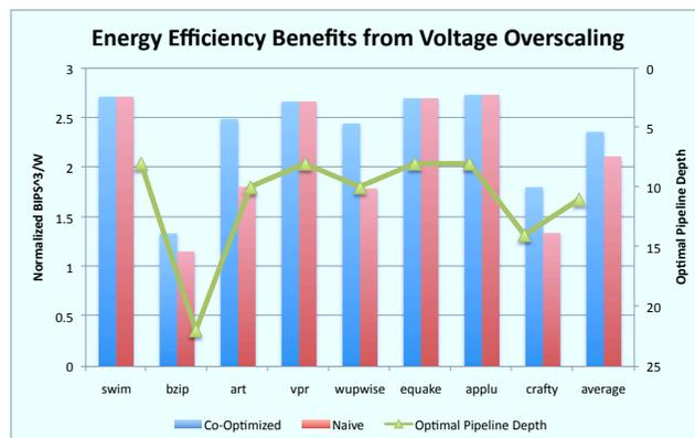
Fig. 8. Simulated results illustrating energy-delay<sup>2</sup> when operating at multiple error rates and pipeline depths. Results are normalized to the energy-efficiency of the optimal non-error resilient design.
