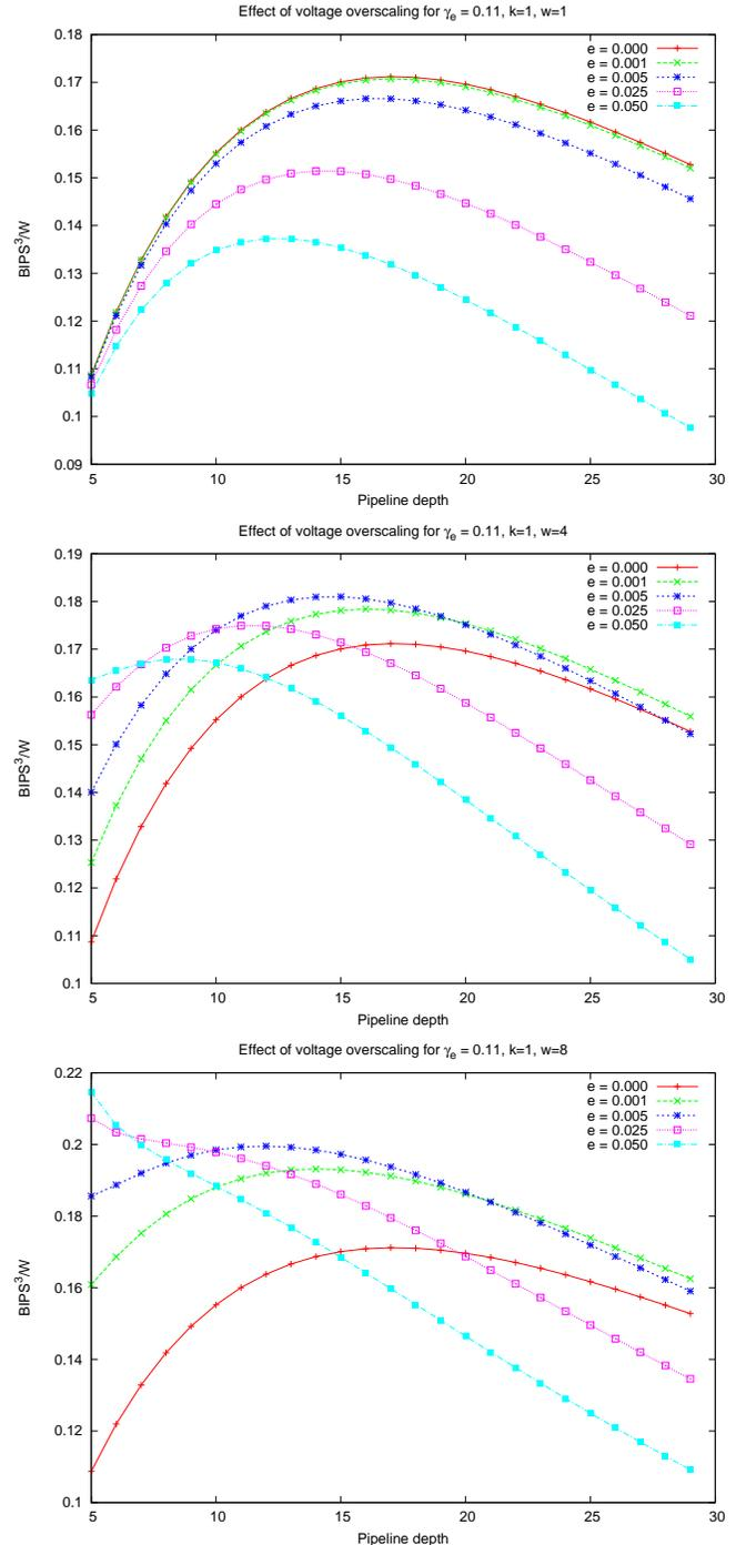
Fig. 2. Error resiliency benefits can be substantial, and are closely tied to both the length of the pipeline and the relationship between error rate and voltage scaling. The figures show error resiliency benefit for different error rate vs voltage scaling relationships. From top to bottom,  $w=1,4,8$ .
