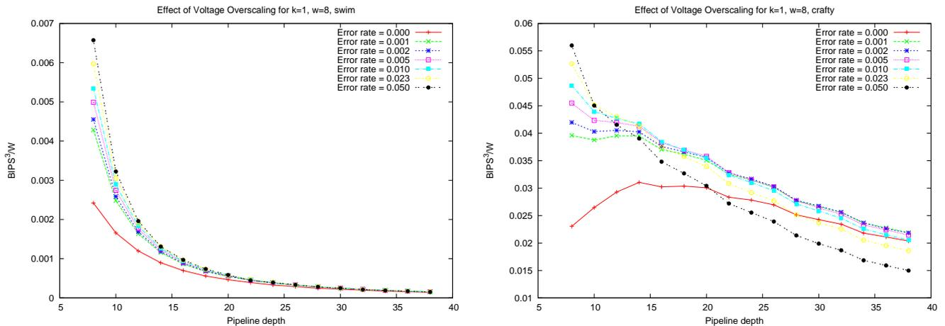
Fig. 7. Simulated results demonstrating the benefits of error resiliency for two benchmarks, SWIM (left) and CRAFTY (right).
