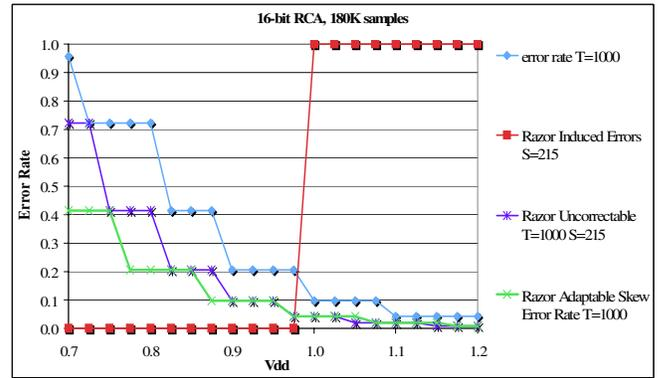
**Figure 10:** Adaptable correction window enhances error protection for aggressive scaling, reducing the number of uncorrectable errors. The technique also increases the usable range for Razor by eliminating false error detections.
