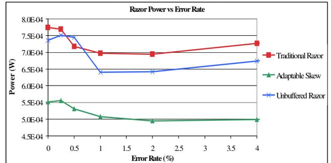
**Figure 11:** The adaptable skew technique reduces both implementation cost and uncorrectable errors, resulting in the ability to correct more errors for the same power or achieve the same correction rate at reduced power.
