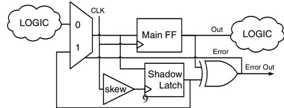
Figure 1: The Razor flip-flop[1].
