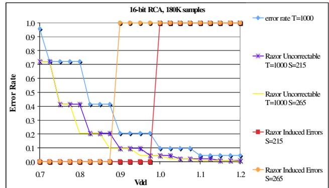
**Figure 7:** The ripple carry adder exhibits a wide range of delay paths, characteristic of a circuit that fails gracefully. Error rate for the circuit increases as supply voltage decreases.
