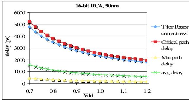
**Figure 8:** The delay characteristics of the Kogge-Stone adder demonstrate its critical wall behavior and unsuitability for aggressive scaling. The wide range of delays for the ripple carry adder demonstrate its capacity to fail gracefully, as well as the large margin for power savings with aggressive scaling.
