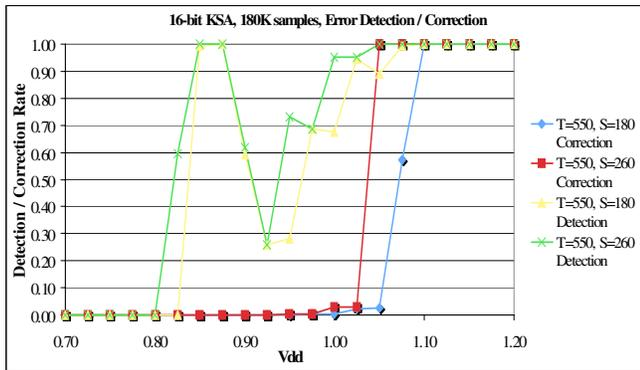
**Figure 6:** Error detection and correction for the KSA.
