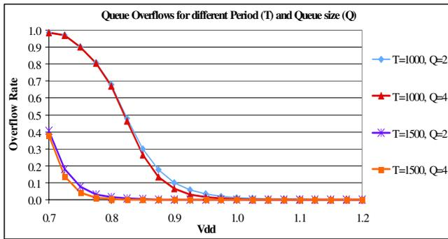
**Figure 13:** Queue overflows remain low when clock period is less than average latency, but increase steeply afterward. This demonstrates that throughput for the decoupled logic is governed by average latency.
