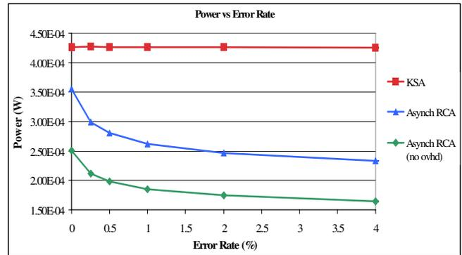
**Figure 14:** Locally asynchronous design allows the RCA to operate at average latency and keep up with the highly optimized KSA. Even with the overhead of logic decoupling, the decoupled RCA consumes less power than the KSA for the same error rate. Also, reliability can be traded for additional power savings due to the graceful failure characteristic of the decoupled design.
