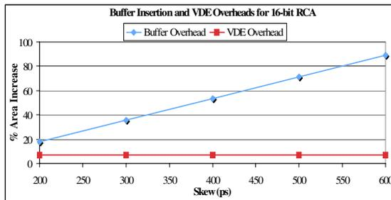
**Figure 9:** As skew increases, the number of uncorrectable errors decreases. However, increased error correction comes at the cost of increased buffering overhead, required to make Razor work when short path constraints are not satisfied. With an adaptable correction window, buffering overhead is eliminated and only a constant overhead is introduced for insertions of VDEs.
