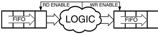
**Figure 3:** FIFOs are used to decouple a pipeline stage. The logic generates an enable signal which communicates externally that computation has finished for the current inputs.
