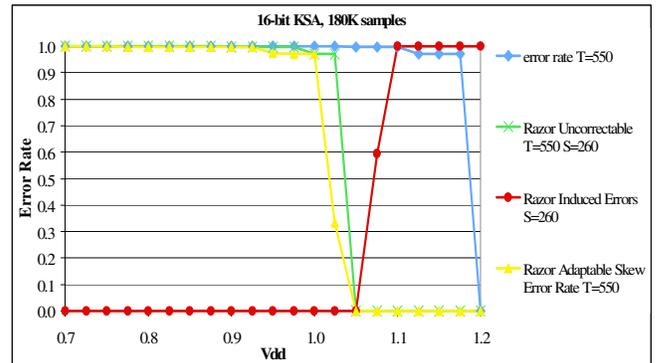
**Figure 12:** Adaptable Correction Window for KSA
