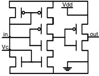
**Figure 2:** The delay of the current starved delay element increases as control voltage ( $V_c$ ) decreases.
