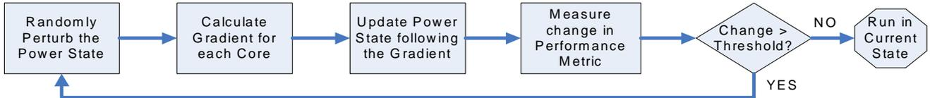
**Figure 5. The gradient ascent approach performs power management locally at each core rather than relying on a global arbiter.**
