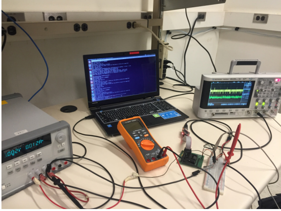
Figure 6: The test setup used to measure peak and average power on a ULP processor (MSP430).
